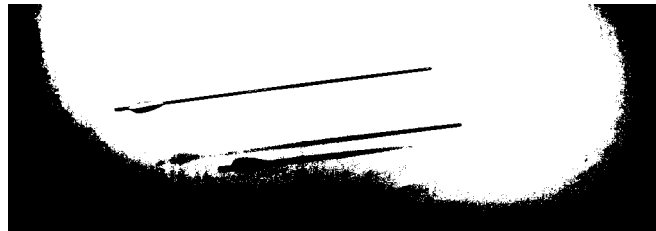
Figure B.2: A single binary image of the flying arrow from the high-speed video camera recordings.
