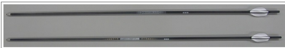
Figure 2.4: Arrows using the two types of shafts, in the upper part an arrow using the A/C/E shaft. In the lower part an arrow using the X10 shaft. Both arrows using the curved SWV vanes.
