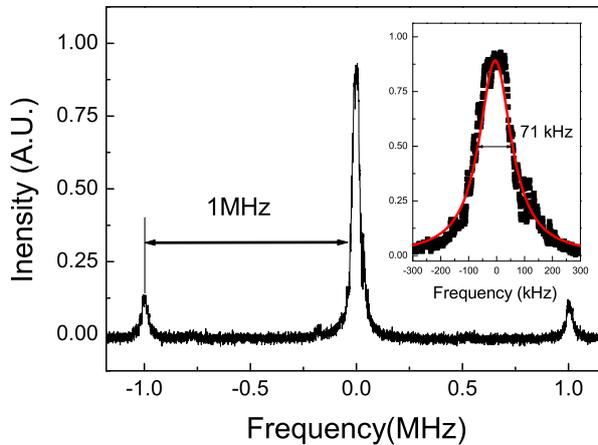
**Figure 3.** (color online) Transmission of the scanned F-P cavity. In the inset, spectrum of the 540 nm light observed with a non-confocal F-P spectrum analyzer. The red curve is the fit with a Lorentzian.
