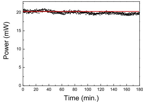
**Figure 2.** (color online) Long-term measurement of the generated 540 nm power.
