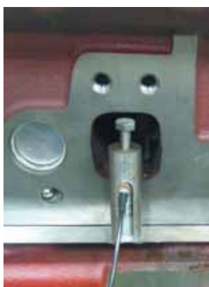
Fig.3 AE sensor attached on the gasket
