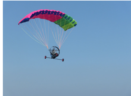
Fig. 1. Photo of UAV-PW during flight.
