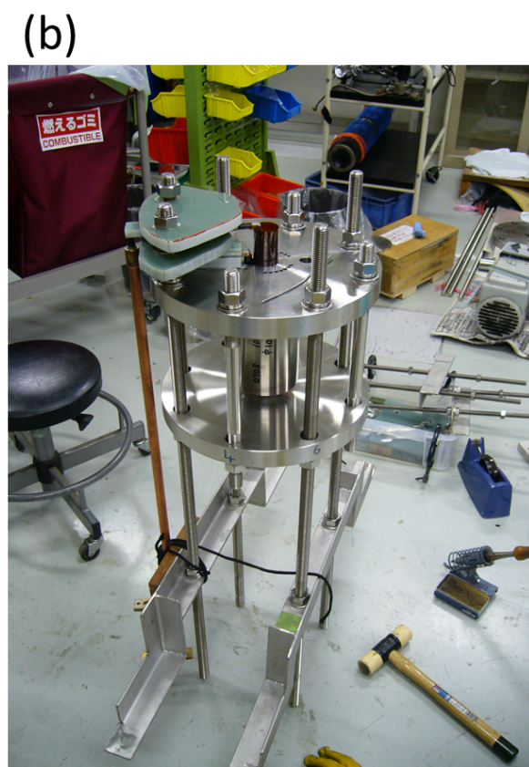
図 2.4: (a) Picture of winding magnet. (b) Magnet after wired electrodes.
