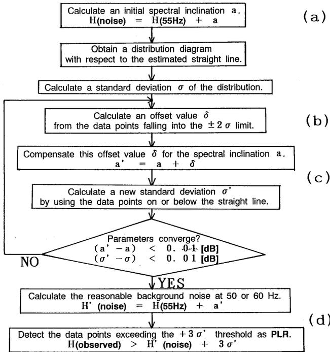
Fig. 2 Flow chart for estimating the real amplitude distribution of the background noise from the observation data which is disturbed by PLR. Steps of this estimation process are illustrated in Fig. 3.
