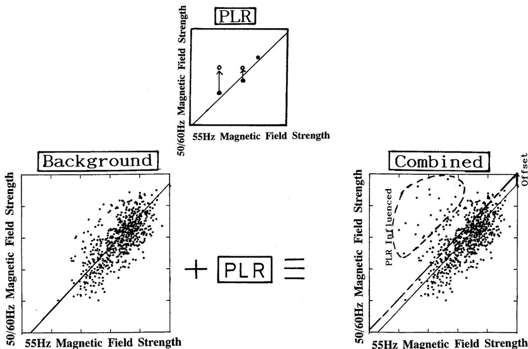
Fig. 1 Expected scheme of the influence of power line radiation (PLR) on background noise.
