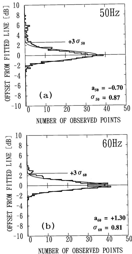
**Fig. 5** Distribution, (a) for 50 Hz, and (b) for 60 Hz, with respect to the fitted line which is estimated by the process as indicated in Fig. 2. The actual distribution is indicated by the histogram with the 0.2 dB bin. The estimated Gaussian distribution curve is shown by the solid curve. The  $+3\sigma$  limit is indicated by the thin line.
