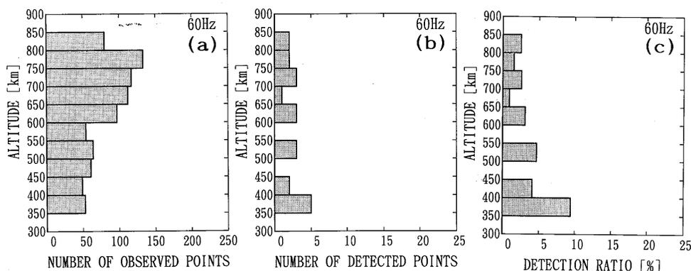
Fig. 9 Altitude dependency, (a) of all of the observed data points, (b) of the detected data points, and (c) of the detection ratio, for 60 Hz.
