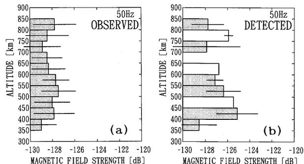
Fig. 10 Average magnetic field strength vs. satellite altitude, (a) for all of the observed data points, and (b) for the detected data points, both for 50 Hz. The horizontal short lines across the top of each bar are the standard deviation of each field strength. Shaded bars in (b) indicate statistically reasonable values.
