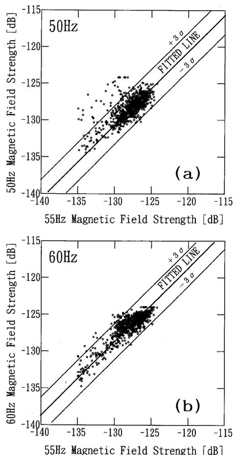
**Fig. 4** (a) Correlation diagram between the field strength at 50 Hz and that at 55 Hz. (b) Correlation diagram between the field strength at 60 Hz and that at 55 Hz. The fitted line indicates the center of the distribution of the background noise, and the  $3\sigma$  lines indicate the  $3\sigma$  limits of the Gaussian distribution with respect to the fitted line. These characteristic parameters of these distributions are calculated by the process described in Fig. 2.
