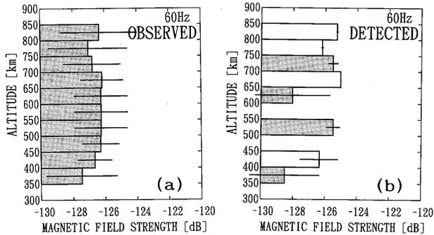
**Fig. 11** Average magnetic field strength vs. satellite altitude, (a) for all of the observed data points, and (b) for the detected data points, both for 60 Hz. The horizontal short lines across the top of each bar are the standard deviation of each field strength. Shaded bars in (b) indicate statistically reasonable values.
