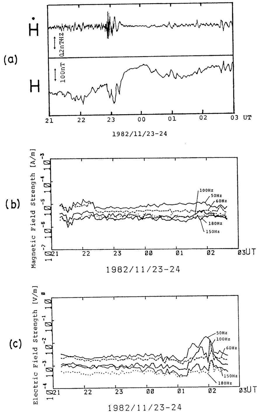
Fig. 4. Strength variations of power line radiations observed on the balloon  $B_{15-2N}$  and their relation to geomagnetic field variations.
