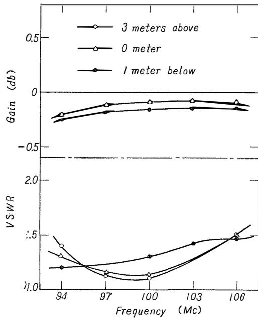
Fig. 11. The results of the measurements of input impedance and gain characteristic by a half wave Folded Dipole for tuned 100 Mc, 3 meters above, 0 meter, 1 meter below the snow surface.
