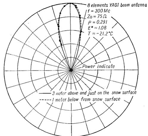
Fig. 8. The horizontal directional pattern of 8 elements YAGI beam antenna for tuned 300 Mc, 3 meters above, 0 meter, 1 meter below the snow surface.
