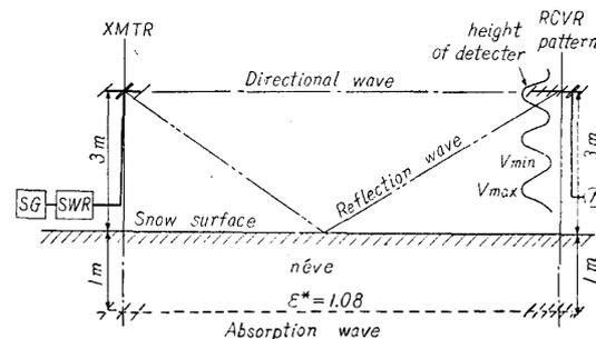
Fig. 13. The measurement of reflection coefficient on the snow surface by height pattern.
