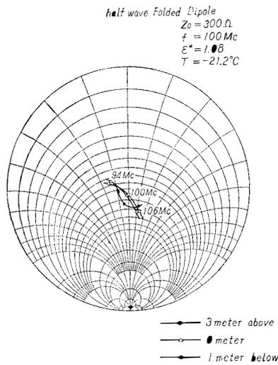
Fig. 9. The impedance characteristics of a half wave Folded Dipole antenna for tuned 100 Mc, 3 meters above, 0 meter, 1 meter below the snow surface.
