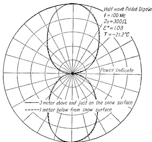
Fig. 7. The horizontal pattern of half wave Folded Dipole antenna for tuned 100 Mc, 3 meters above, 0 meter, 1 meter below the snow surface.
