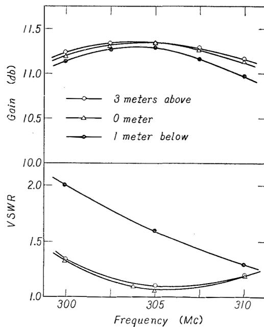
Fig. 12. The results of the measurements of input impedance and gain characteristic by a 8 elements YAGI beam antenna for tuned 300 Mc, 3 meters above, 0 meter, 1 meter below the snow surface.
