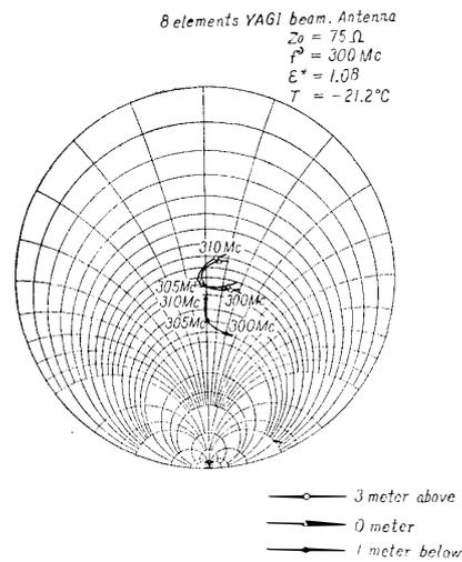
Fig. 10. The impedance characteristics of a 8 elements YAGI beam antenna for tuned 300 Mc, 3 meters above, 0 meter 1 meter below the snow surface.
