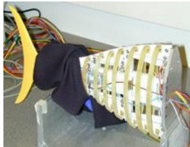
Fig. 1.20 Tail of robot using SMA [74].
