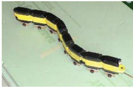
Fig. 1.7 Snake-like robot AmphiBot developed by EPFL [33].
