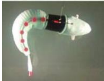
Fig. 1.8 Soft robotic fish developed by MIT [53].
