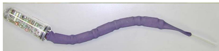
Fig. 1.10 Undulatory robotic lamprey using SMA [60].
