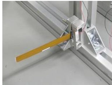
Fig. 3.11 Prototype of beam structure.
