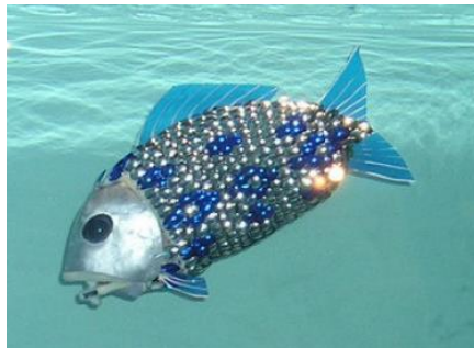
Fig. 1.6 Biomimetic robotic fish used in detection of pollutants from Essex University [34].
