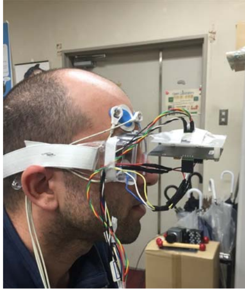
Figure 3.5 Experimental setup when the Doppler sensor was attached to a pair of glasses.
