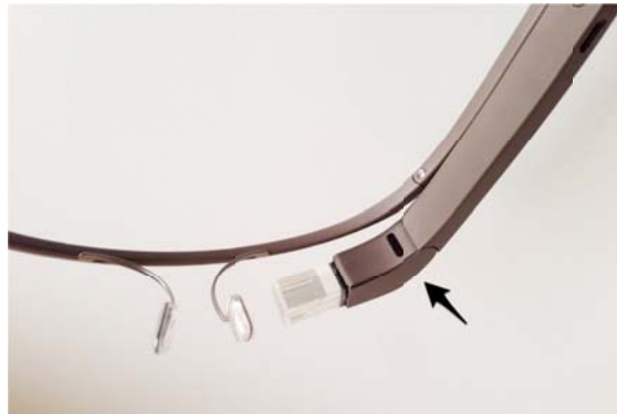
Figure 1.2 Infrared proximity sensor built into Google Glass (Ishimaru et al., 2014).
