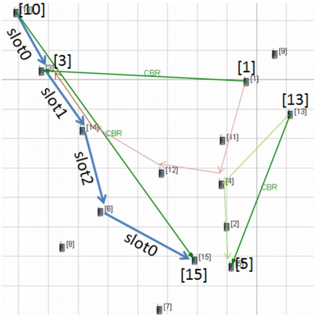
Figure 45 Topology and corresponding time slot assignment in simulation I.
