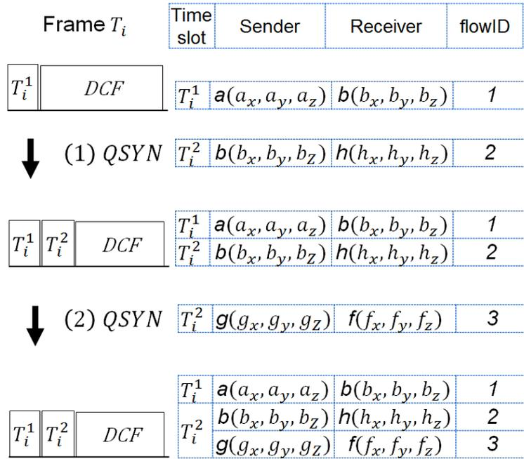
Figure 36 Add a new time slot to the frame according the QSYN message.
