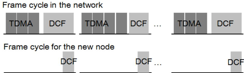
Figure 79 Setting of frame at new node.
