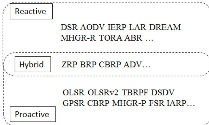
Figure 17 Routing Protocols in wireless ad hoc networks.
