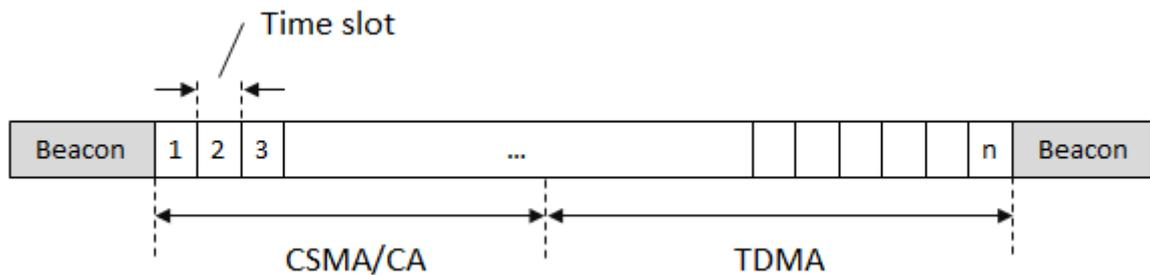
Figure 16 Superframe Structure of CSMA/CA-TDMA.
