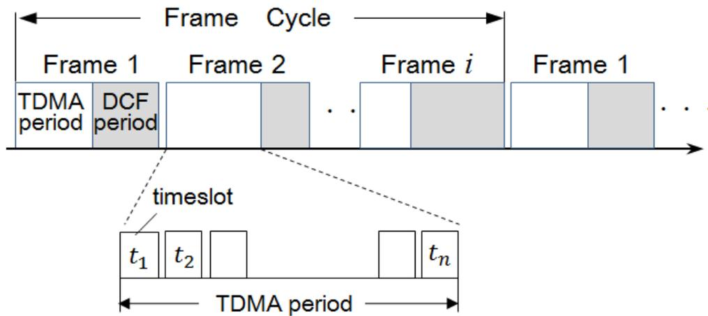
Figure 21 Structure of time frame in proposed scheme.
