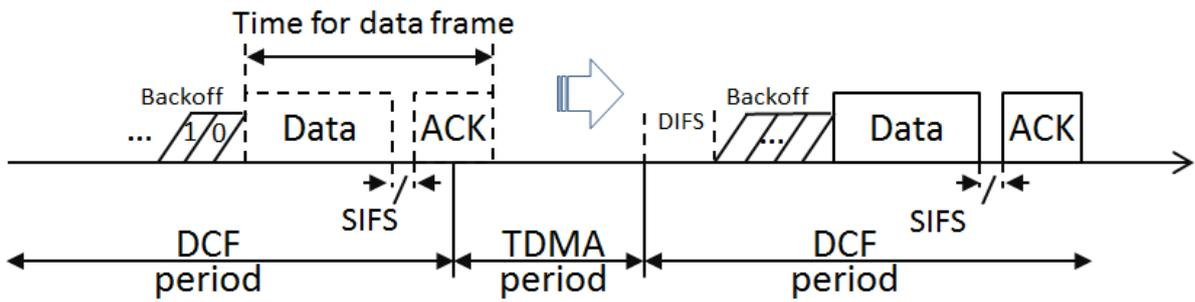
Figure 38 An example for controlling the data transfer at the end of DCF period.
