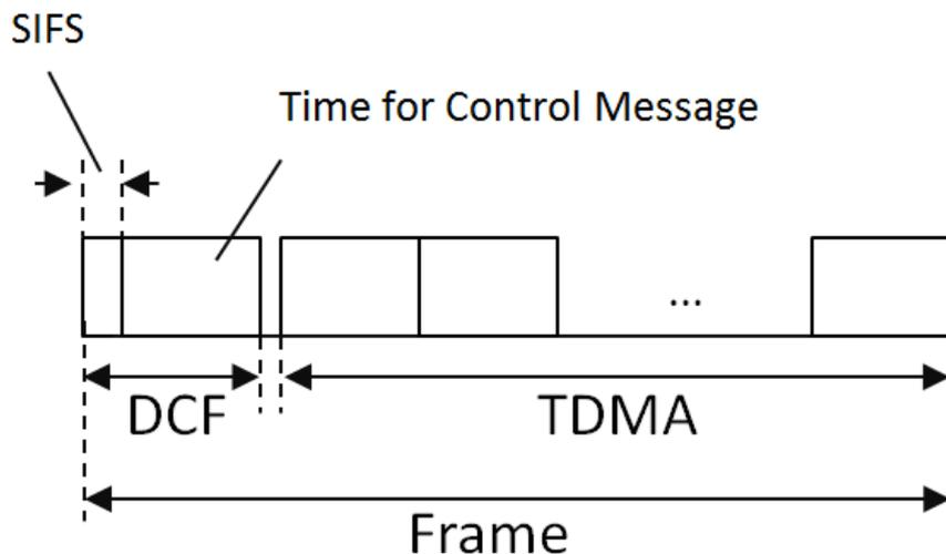
Figure 22 The minimum length of DCF period in a frame.
