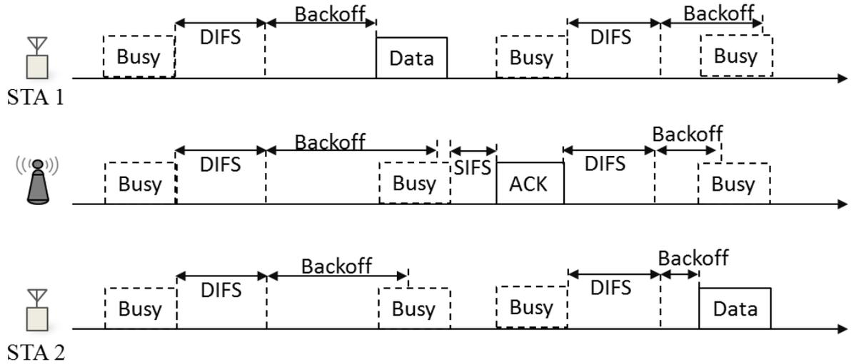
Figure 7 Backoff Mechanism in DCF protocol.
