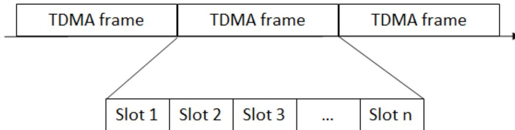
Figure 13 TDMA Frame Structure.
