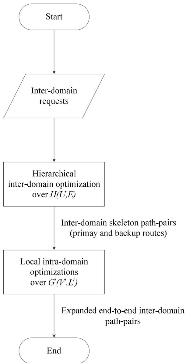
**Figure 6.1:** Flowchart of two-phase lightpath provisioning.
