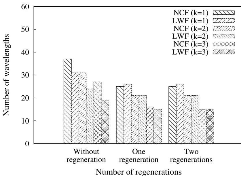
**Figure 5.19:** Number of required wavelengths of the heuristic RWA scheme with three MCLS nodes for European COST 239 network with 200 requested lightpaths.
