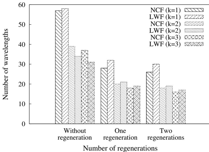
**Figure 5.14:** Number of required wavelengths of the heuristic RWA scheme with one MCLS node for Synthetic network with 200 requested lightpaths.
