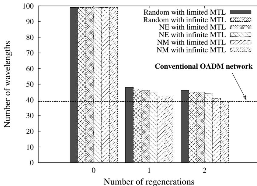
**Figure 3.11:** Number of required wavelengths with the heuristic RWA scheme (different requested lightpath selection policies) for European COST 239 network with 300 requested lightpaths.
