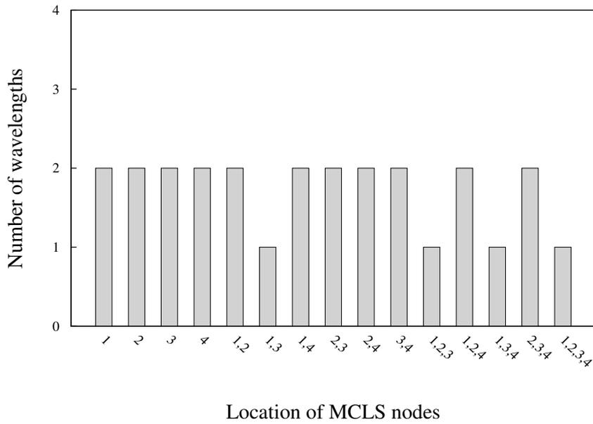
**Figure 4.8:** Comparison of number of wavelengths in each possible MCLS nodes under the ILP approach without regeneration for Topology 3.
