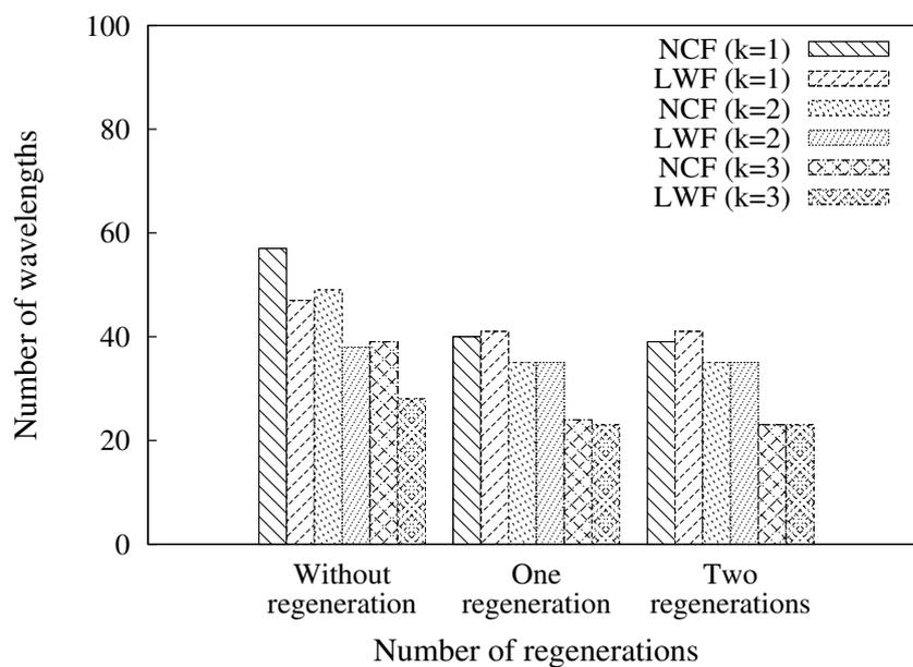
**Figure 5.28:** Number of required wavelengths of the heuristic RWA scheme with three MCLS nodes for European COST 239 network with 300 requested lightpaths.
