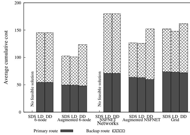
Figure 6.3: Average cumulative cost ( $C_{ij,km}^G = C_{i,jk}^L = 8$  and  $r_n = 1$ ).
