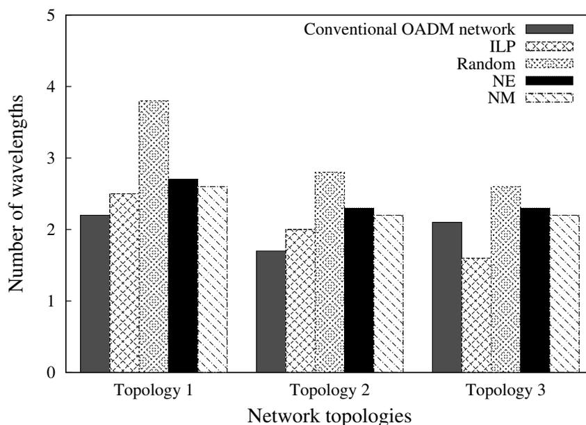
**Figure 3.6:** Comparison of the number of required wavelengths of ILP approach and heuristic RWA scheme with one regeneration.
