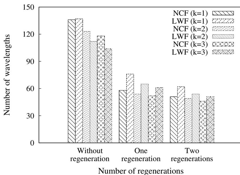
**Figure 5.29:** Number of required wavelengths of the heuristic RWA scheme with one MCLS node for U.S. long distance network with 300 requested lightpaths.
