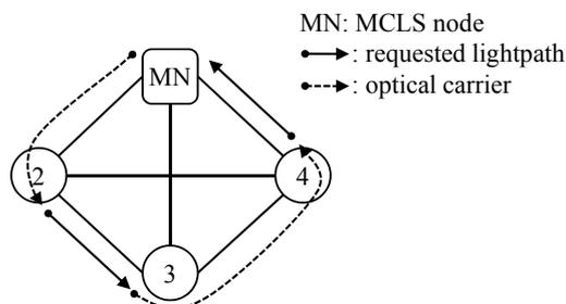
**Figure 2.2:** Lightpath establishment with optical carrier regeneration.
