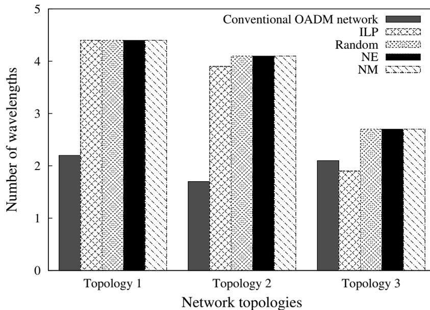
**Figure 3.5:** Comparison of the number of required wavelengths of ILP approach and heuristic RWA scheme without regeneration.
