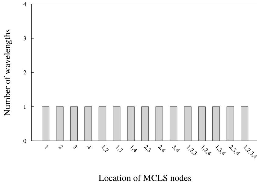
**Figure 4.10:** Comparison of number of wavelengths in each possible MCLS nodes under the ILP approach with two regenerations for Topology 3.
