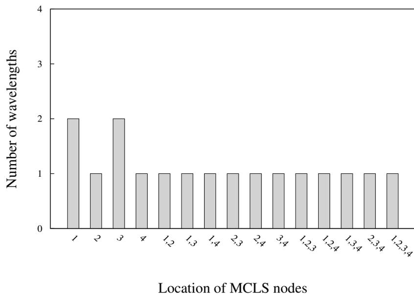
**Figure 4.6:** Comparison of number of wavelengths in each possible MCLS nodes under the ILP approach with one regeneration for Topology 2.
