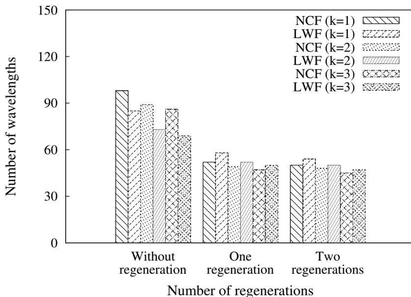
**Figure 5.30:** Number of required wavelengths of the heuristic RWA scheme with two MCLS nodes for U.S. long distance network with 300 requested lightpaths.
