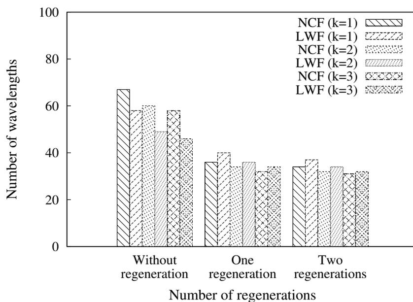
**Figure 5.21:** Number of required wavelengths of the heuristic RWA scheme with two MCLS nodes for U.S. long distance network with 200 requested lightpaths.
