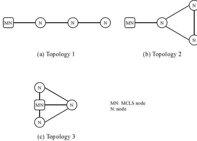
**Figure 3.3:** Network topologies for comparison of ILP approach and heuristic RWA scheme.
