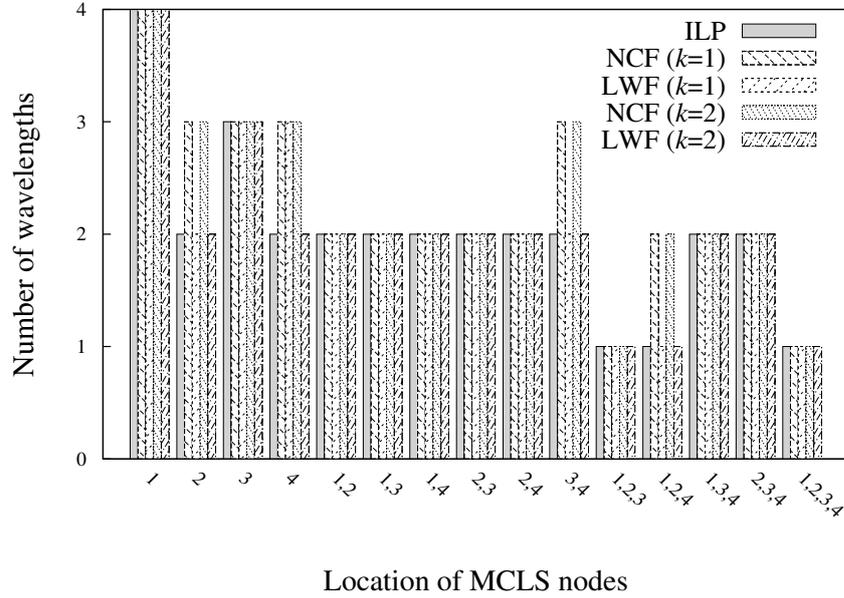
**Figure 5.7:** Comparison of the number of wavelengths required under the ILP approach and heuristic RWA scheme without regeneration for Topology 2.
