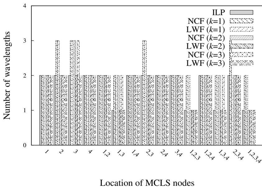
**Figure 5.10:** Comparison of the number of wavelengths required under the ILP approach and heuristic RWA scheme without regeneration for Topology 3.
