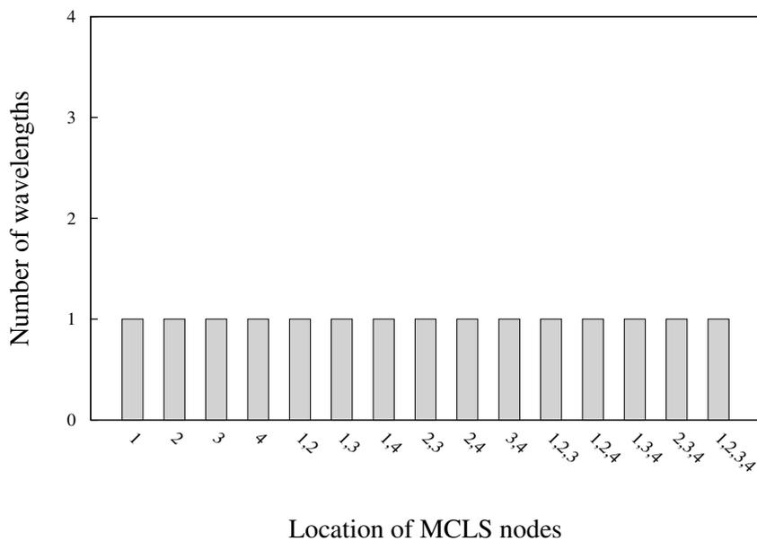
**Figure 4.9:** Comparison of number of wavelengths in each possible MCLS nodes under the ILP approach with one regeneration for Topology 3.
