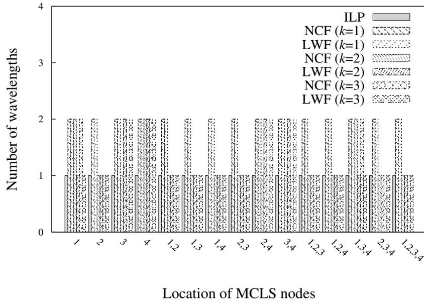
**Figure 5.11:** Comparison of the number of wavelengths required under the ILP approach and heuristic RWA scheme with one regeneration for Topology 3.
