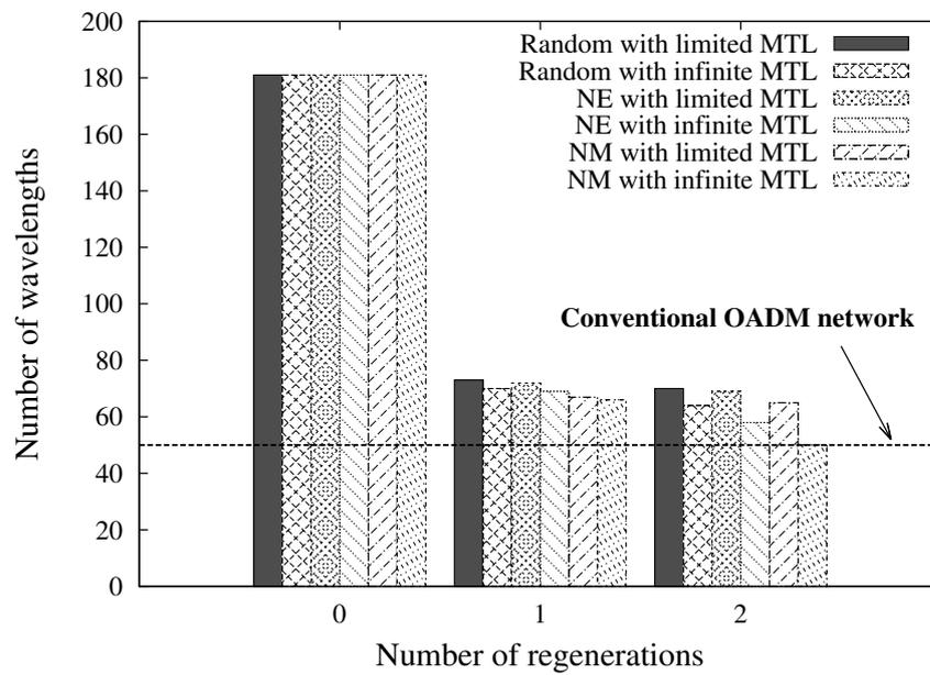
**Figure 3.13:** Number of required wavelengths with the heuristic RWA scheme (different requested lightpath selection policies) for U.S. long distance network with 300 requested lightpaths.
