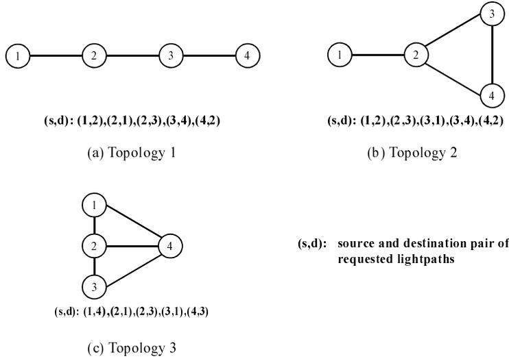
**Figure 4.1:** Network topologies for comparison of ILP approach and heuristic RWA scheme.
