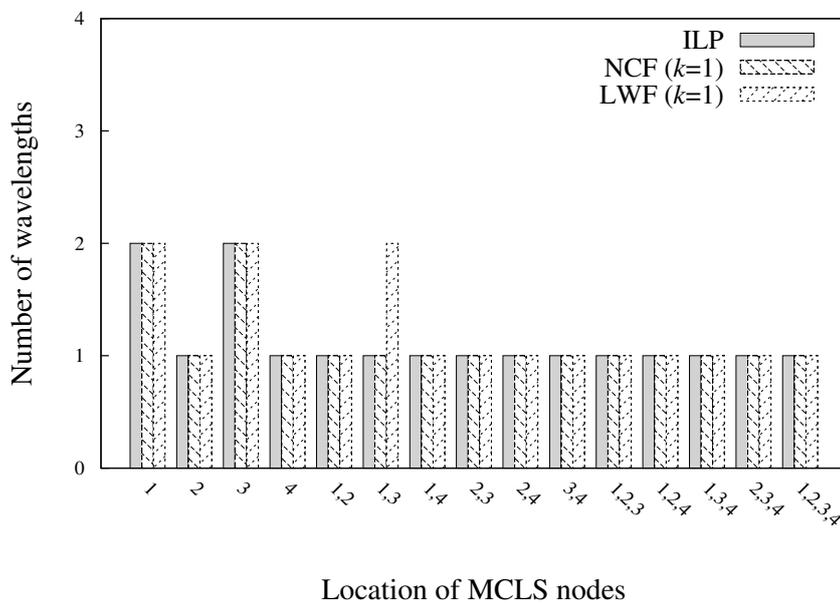
**Figure 5.6:** Comparison of the number of wavelengths required under the ILP approach and heuristic RWA scheme with two regenerations for Topology 1.
