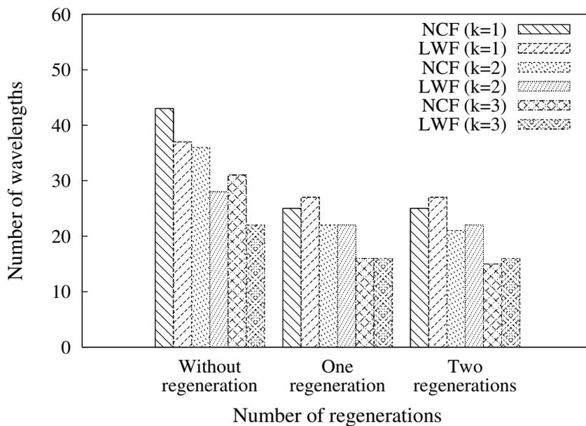
**Figure 5.18:** Number of required wavelengths of the heuristic RWA scheme with two MCLS nodes for European COST 239 network with 200 requested lightpaths.
