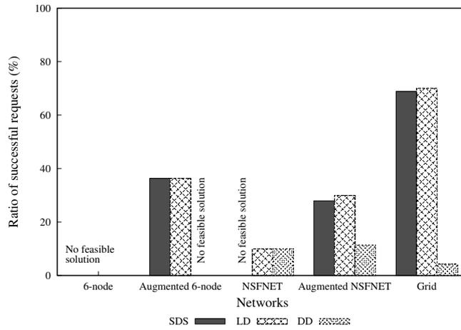
**Figure 6.9:** Successful request ratio ( $C_{ij,km}^G = C_{i,jk}^L = 8$  and  $r_n = 16$ ).
