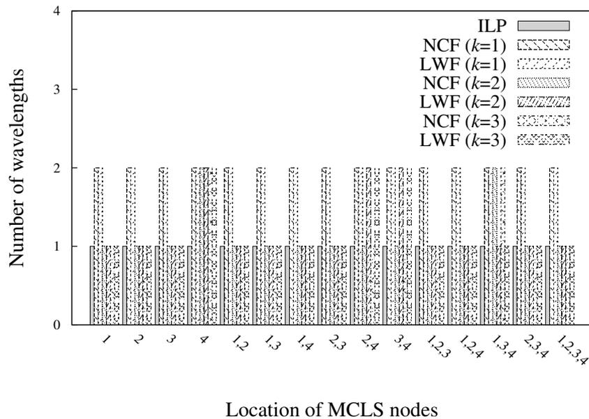
**Figure 5.12:** Comparison of the number of wavelengths required under the ILP approach and heuristic RWA scheme with two regenerations for Topology 3.
