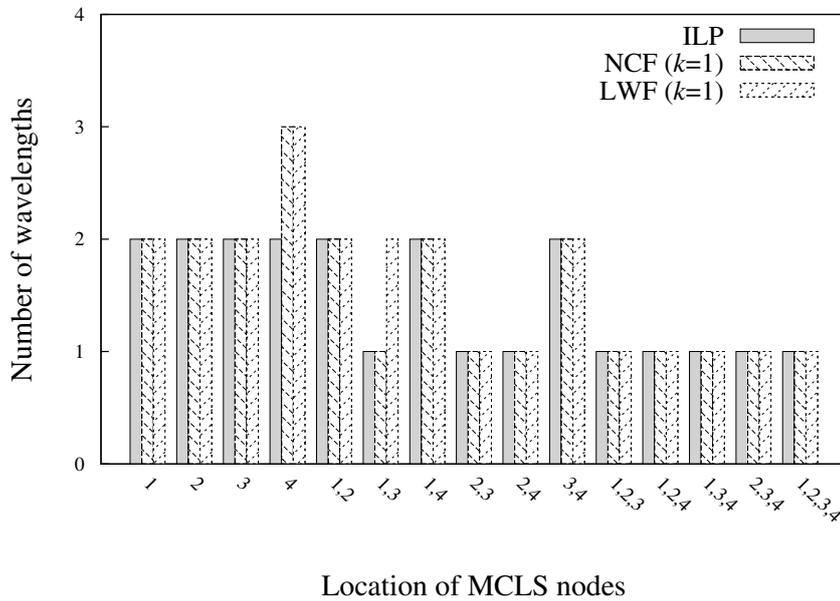
**Figure 5.5:** Comparison of the number of wavelengths required under the ILP approach and heuristic RWA scheme with one regeneration for Topology 1.
