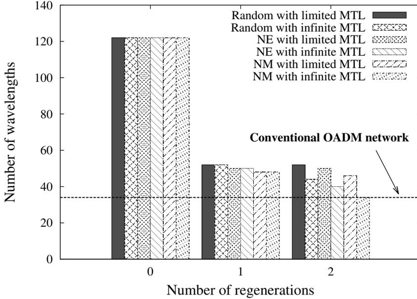
**Figure 3.12:** Number of required wavelengths with the heuristic RWA scheme (different requested lightpath selection policies) for U.S. long distance network with 200 requested lightpaths.
