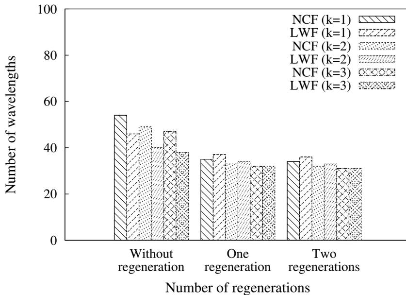
**Figure 5.22:** Number of required wavelengths of the heuristic RWA scheme with three MCLS nodes for U.S. long distance network with 200 requested lightpaths.
