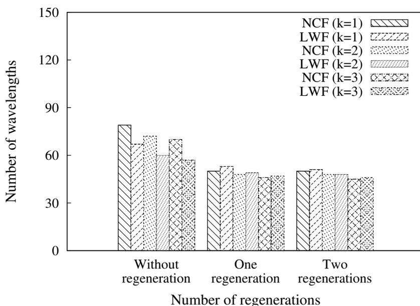
**Figure 5.31:** Number of required wavelengths of the heuristic RWA scheme with three MCLS nodes for U.S. long distance network with 300 requested lightpaths.
