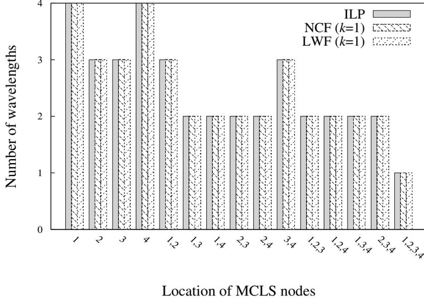
**Figure 5.4:** Comparison of the number of wavelengths required under the ILP approach and heuristic RWA scheme without regeneration for Topology 1.
