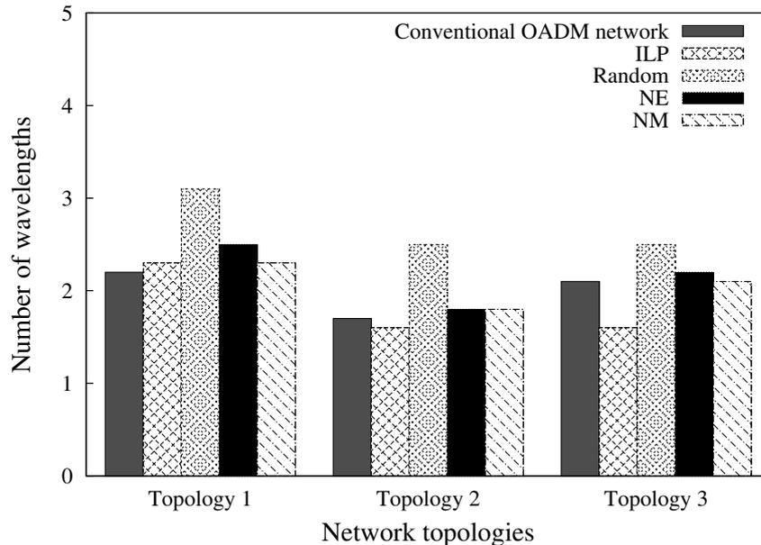
**Figure 3.7:** Comparison of the number of required wavelengths of ILP approach and heuristic RWA scheme with two regenerations.
