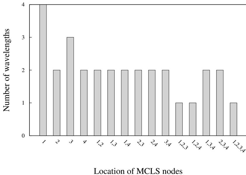
**Figure 4.5:** Comparison of number of wavelengths in each possible MCLS nodes under the ILP approach without regeneration for Topology 2.
