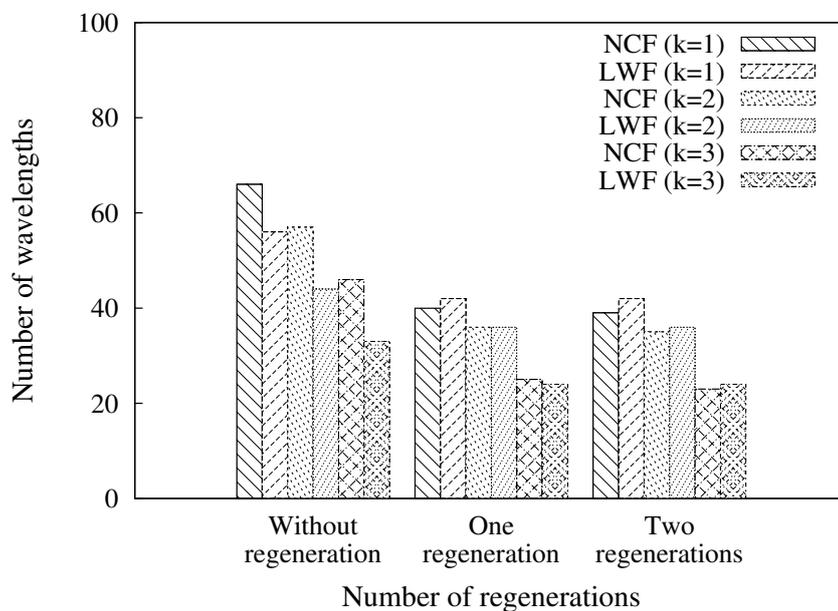
**Figure 5.27:** Number of required wavelengths of the heuristic RWA scheme with two MCLS nodes for European COST 239 network with 300 requested lightpaths.
