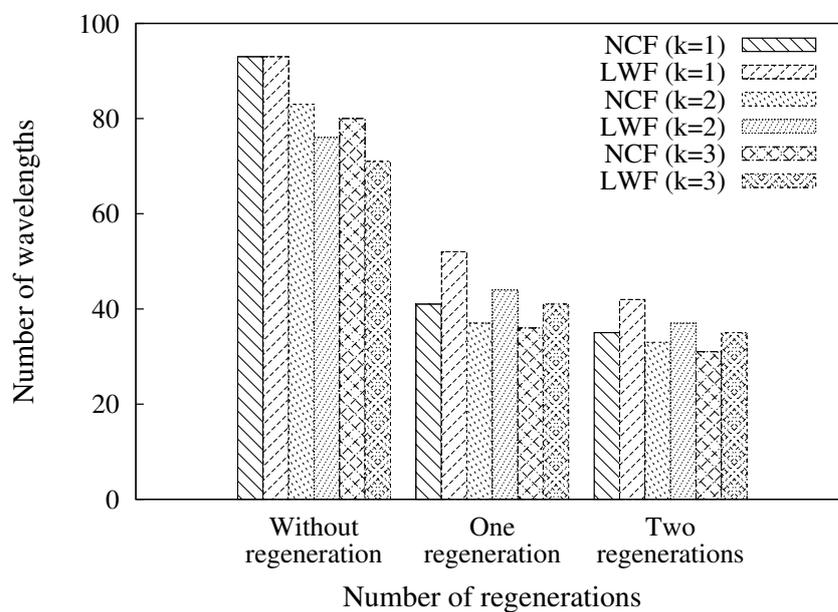
**Figure 5.20:** Number of required wavelengths of the heuristic RWA scheme with one MCLS node for U.S. long distance network with 200 requested lightpaths.
