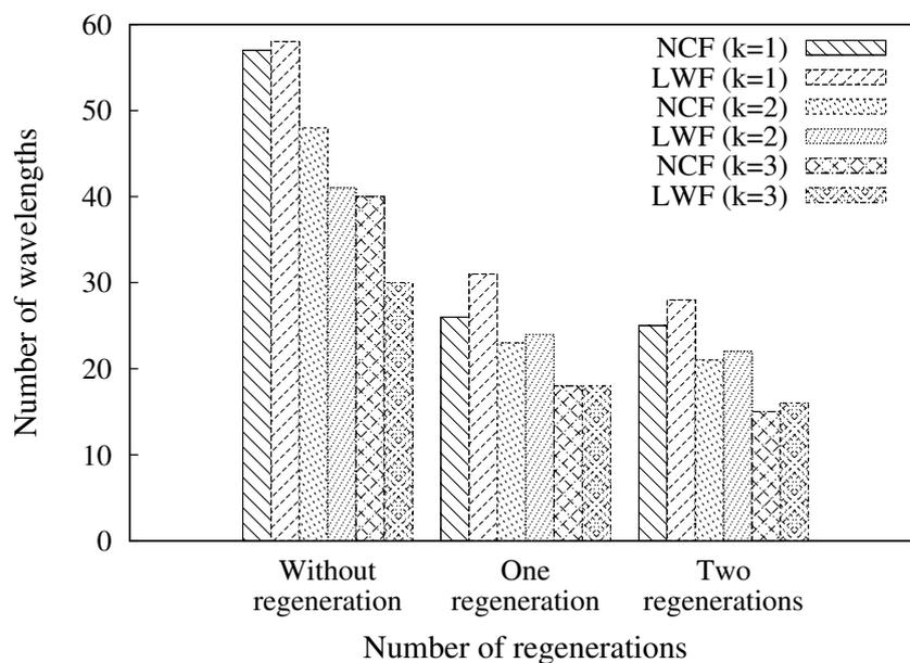
**Figure 5.17:** Number of required wavelengths of the heuristic RWA scheme with one MCLS node for European COST 239 network with 200 requested lightpaths.
