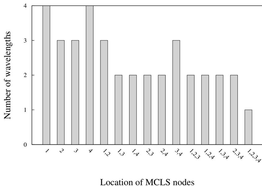
**Figure 4.2:** Comparison of number of wavelengths in each possible MCLS nodes under the ILP approach without regeneration for Topology 1.
