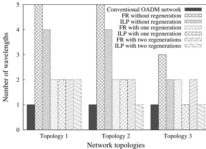
**Figure 2.5:** Comparison of the number of required wavelengths of FR scheme and ILP approach.
