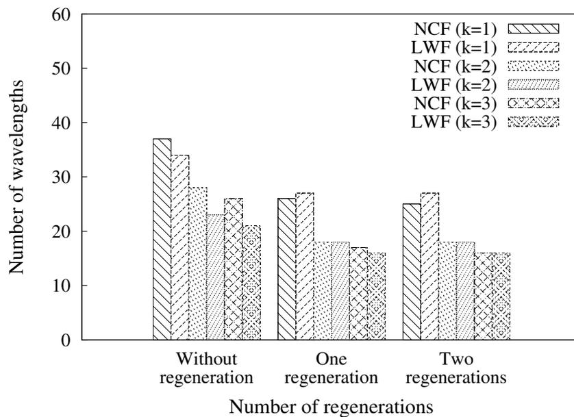
**Figure 5.16:** Number of required wavelengths of the heuristic RWA scheme with three MCLS nodes for Synthetic network with 200 requested lightpaths.
