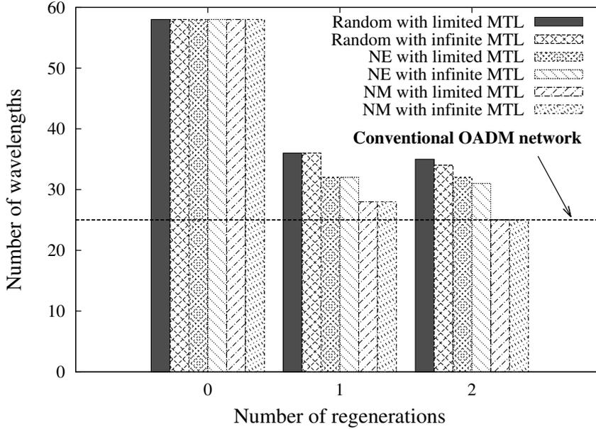
**Figure 3.8:** Number of required wavelengths with the heuristic RWA scheme (different requested lightpath selection policies) for Synthetic network with 200 requested lightpaths.
