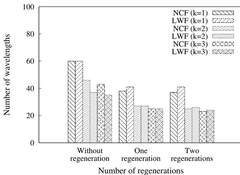
**Figure 5.24:** Number of required wavelengths of the heuristic RWA scheme with two MCLS nodes for Synthetic network with 300 requested lightpaths.
