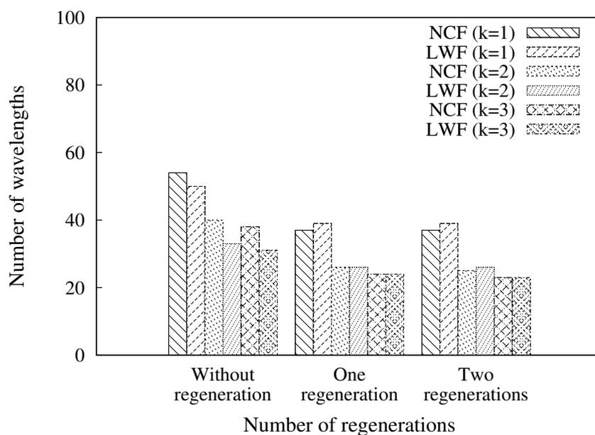
**Figure 5.25:** Number of required wavelengths of the heuristic RWA scheme with three MCLS nodes for Synthetic network with 300 requested lightpaths.
