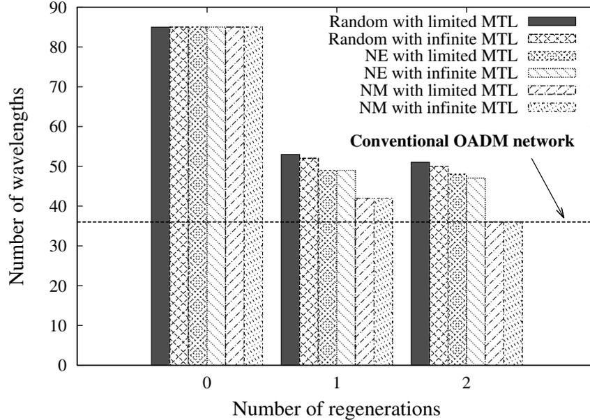
**Figure 3.9:** Number of required wavelengths with the heuristic RWA scheme (different requested lightpath selection policies) for Synthetic network with 300 requested lightpaths.
