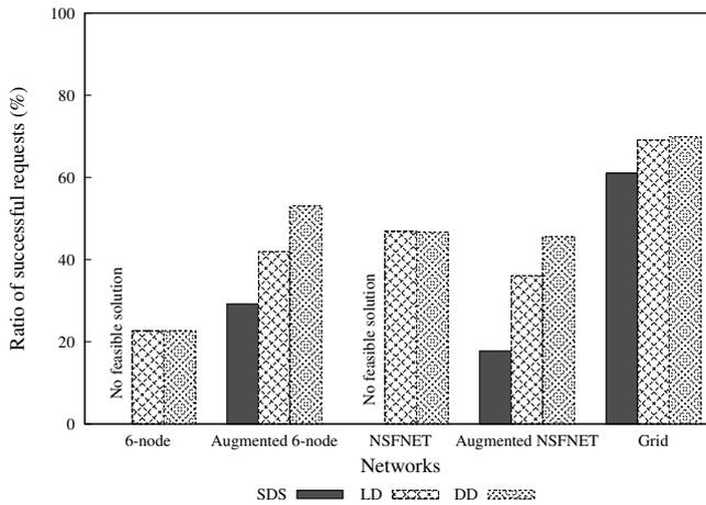
**Figure 6.17:** Successful request ratio ( $C_{ij,km}^G = 2C_{i,jk}^L = 16$  and  $r_n = 16$ ).
