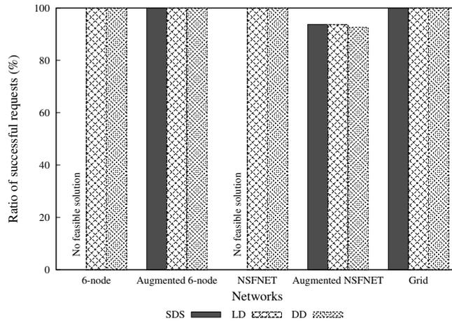
**Figure 6.5:** Successful request ratio ( $C_{ij,km}^G = C_{i,jk}^L = 8$  and  $r_n = 1$ ).
