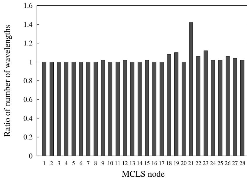
**Figure 3.16:** Comparison of number of wavelengths in each MCLS node for U.S. long distance network with 300 requested lightpaths.
