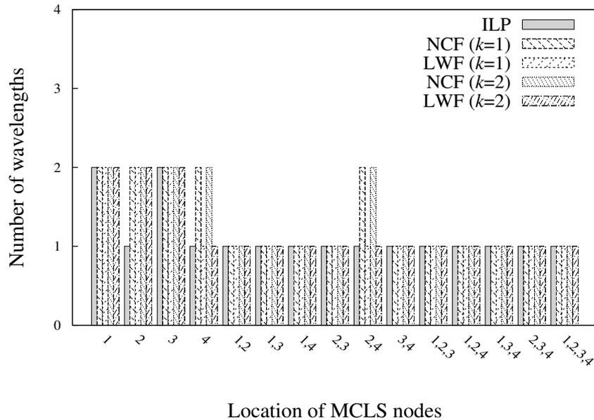
**Figure 5.8:** Comparison of the number of wavelengths required under the ILP approach and heuristic RWA scheme with one regeneration for Topology 2.
