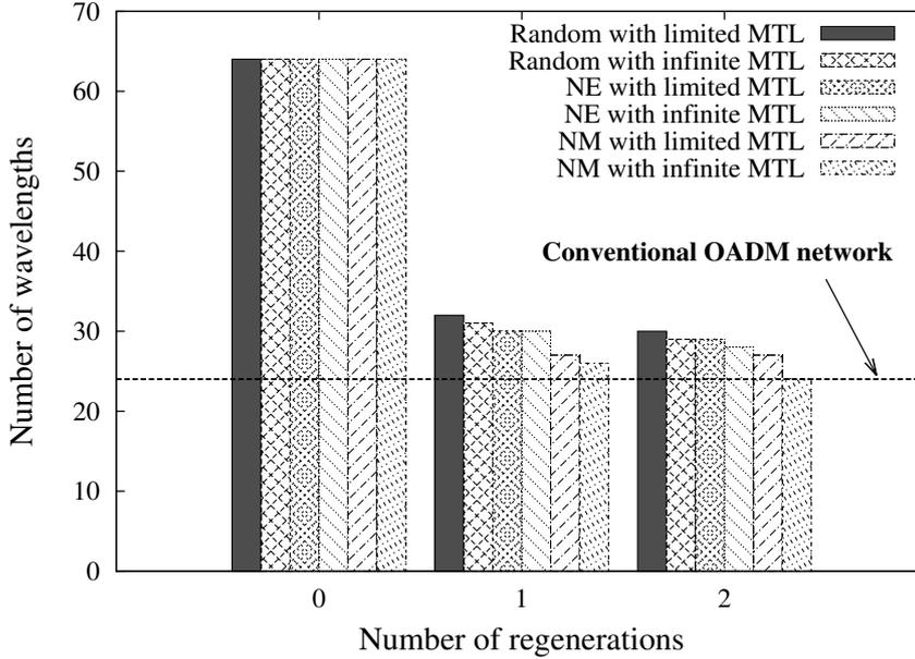
**Figure 3.10:** Number of required wavelengths with the heuristic RWA scheme (different requested lightpath selection policies) for European COST 239 network with 200 requested lightpaths.
