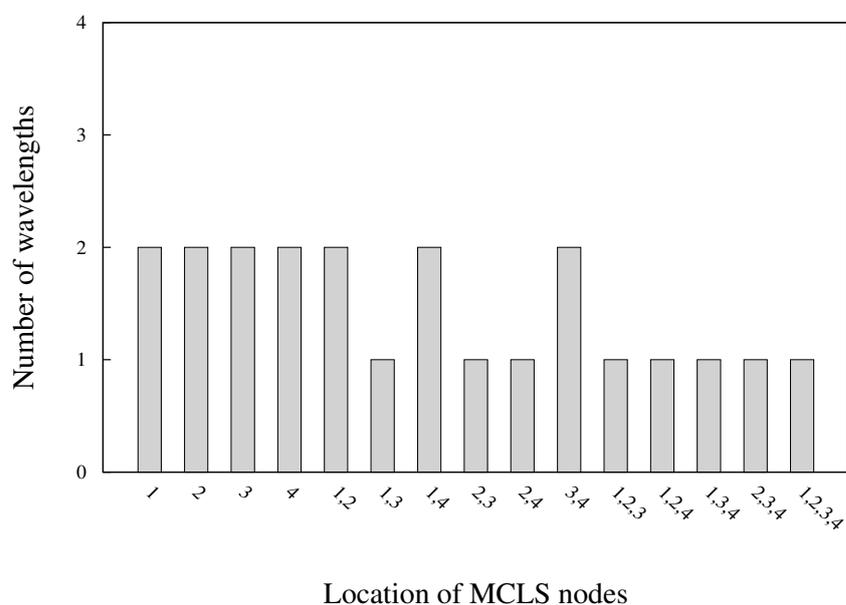
**Figure 4.3:** Comparison of number of wavelengths in each possible MCLS nodes under the ILP approach with one regeneration for Topology 1.
