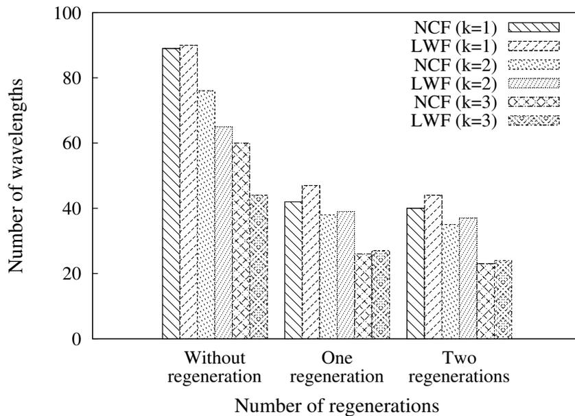
**Figure 5.26:** Number of required wavelengths of the heuristic RWA scheme with one MCLS node for European COST 239 network with 300 requested lightpaths.
