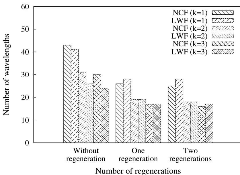
**Figure 5.15:** Number of required wavelengths of the heuristic RWA scheme with two MCLS nodes for Synthetic network with 200 requested lightpaths.
