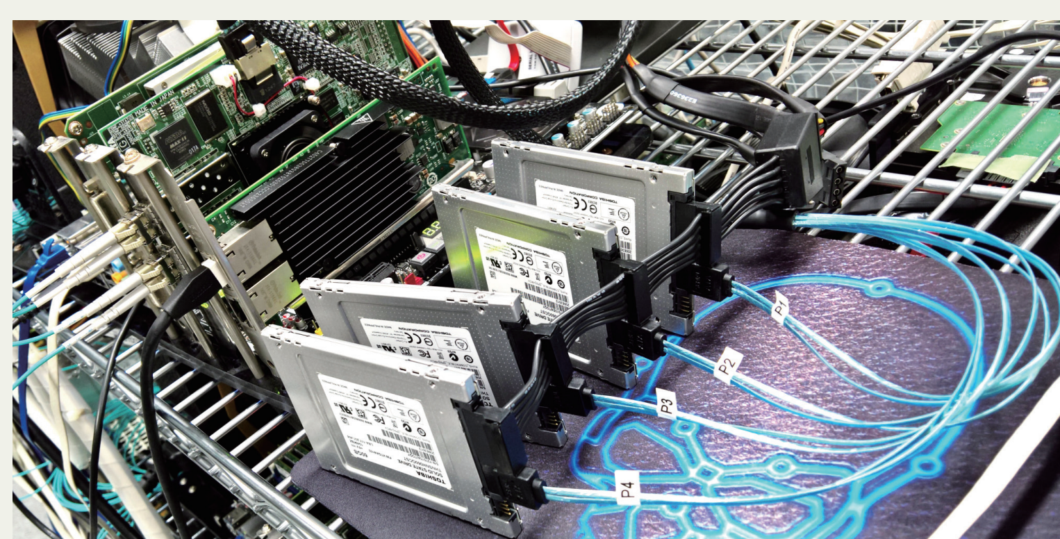
FPGA Board [APX-7142 改] ALTERA StratixV-GX 5SGXMA3K1F40C2N DRAM DDR3 2.0GB SSD 60GB*4(RAID0)
