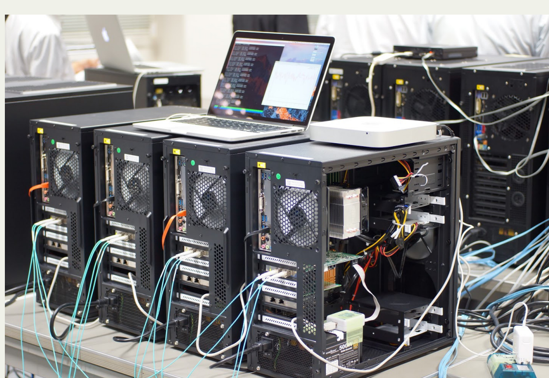
Computing Node Xeon E5-2630 6C/12T 2.6GHz DRAM DDR3 16GB SSD 960GB *2 (RAID0)
