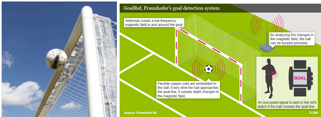
Figure 2.18: GoalRef: Officiating system using magnetic Fields
