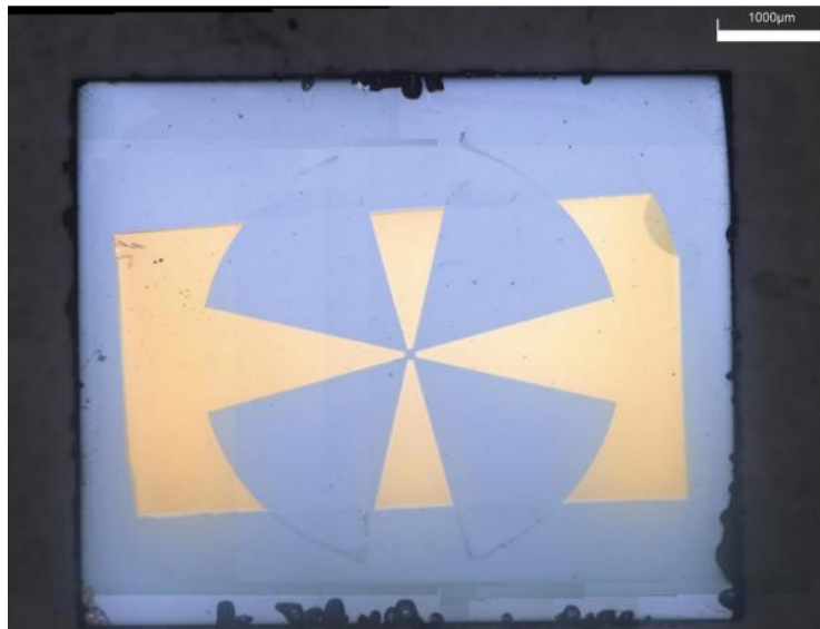
Figure 3.7 AuGe electrodes on sample for photocurrent-voltage measurement.
