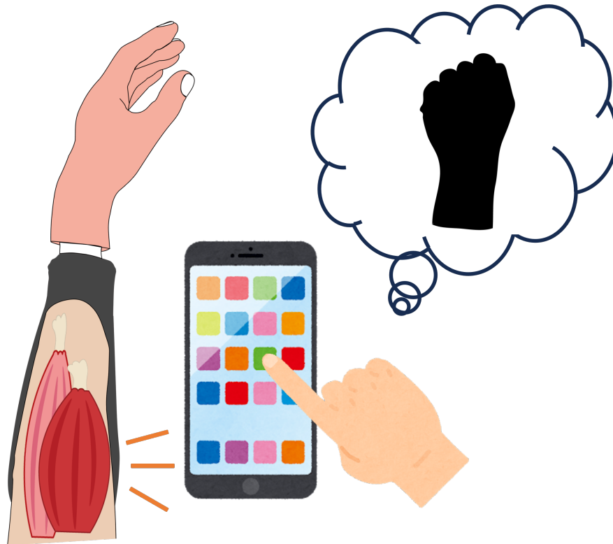
Fig.2.13: Labeling process. The user must press a button corresponding to the desired movement when performing specific muscle activities, thus labeling the signal.
