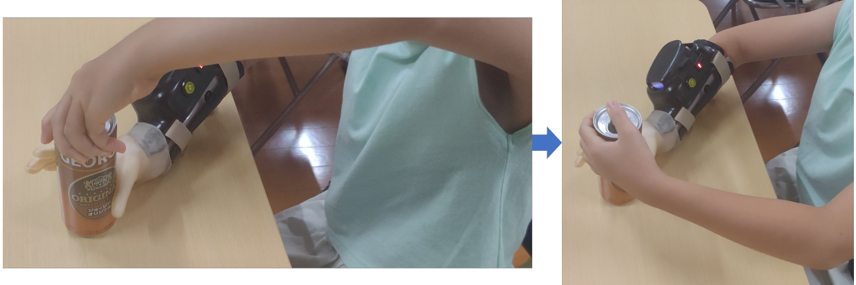
Fig.6.11: Opening a can. The can was held with the MPH, and the stay-on-tab was opened using the fingers of the non-disabled hand.
