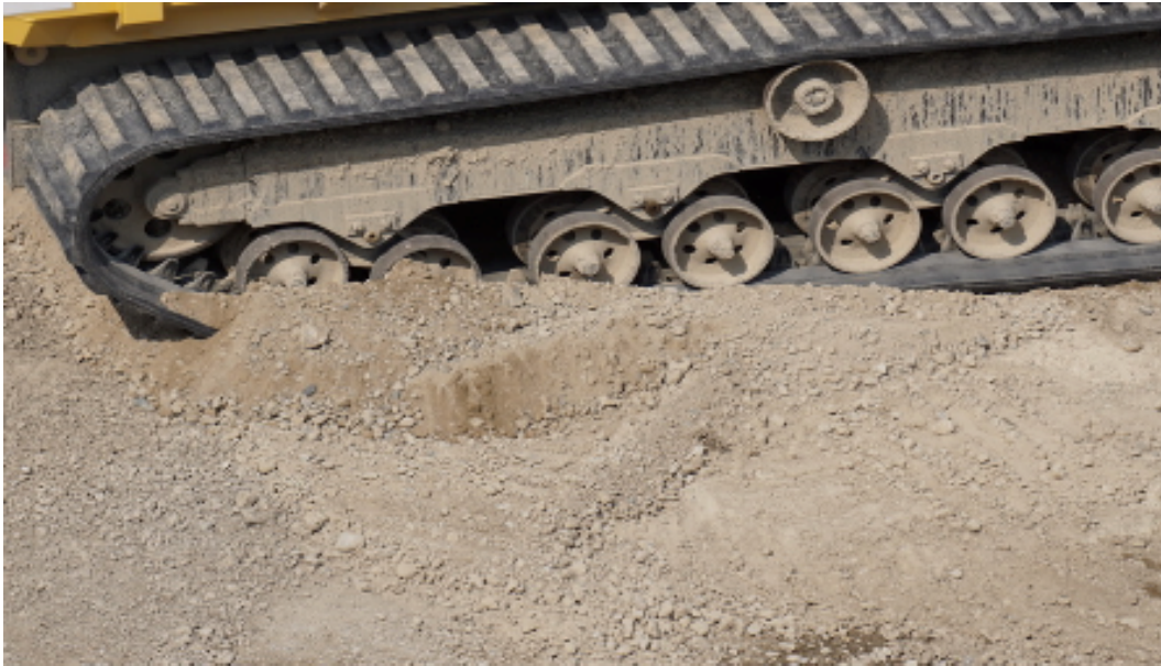
Fig. 3.12: Gravel built up by the crawler of the dump as the crawler rotates in the counterclockwise direction.
