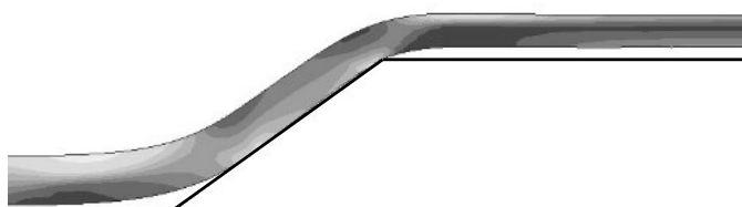
(c) Plug diameter D_p = 38 mm, Half-angle \alpha = 36^\circ , Overshoot g_o = 0.47 mm
