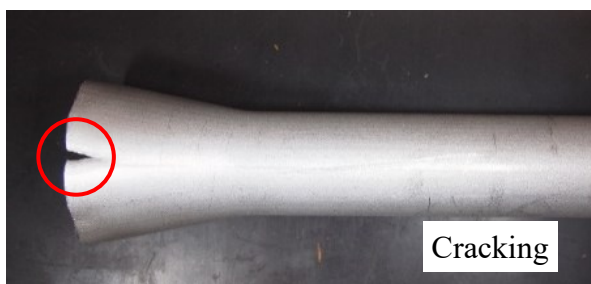
Fig. 2.2.4 Type of flaring defects
