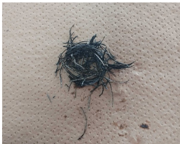
Fig. 2.5.3 Shavings generated on wrinkling (STKM13C Experiment, Half-angle \alpha = 48^\circ , Plug diameter D_p = 30 mm)
