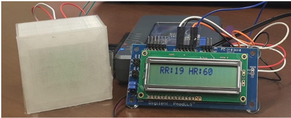
Figure 5.7: Vital sign detection system implemented on FPGA myRIO kit
