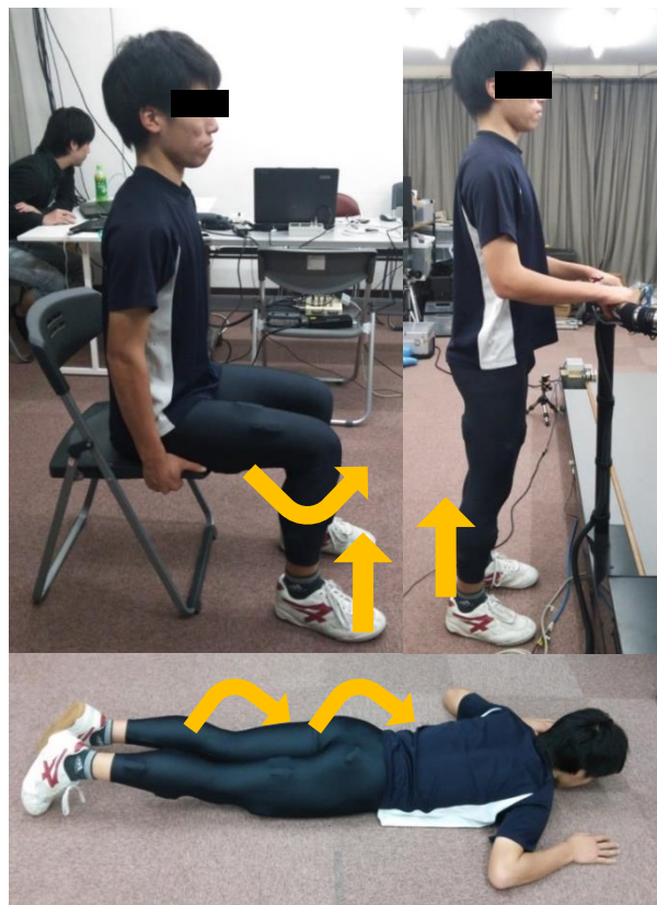
Fig. 2-2 Posture of subjects during MVC (upper left: knee extension and ankle dorsiflexion, upper right: ankle plantar flexion, bottom: hip extension and knee flexion)
