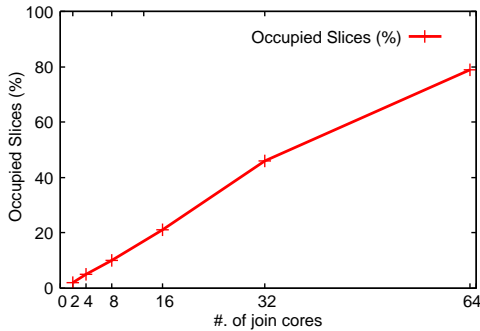
Fig. 11. Overall slice usage of the implemented circuit on a Virtex-6 XC6VLX240T-1 for each of the six different configurations.
