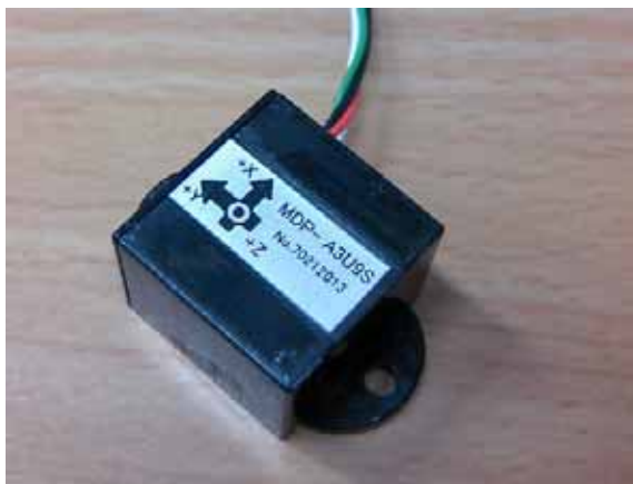
Fig. 6.10:3D motion sensor composed of gyro sensor, acceleration sensor and geomagnetic sensor.
