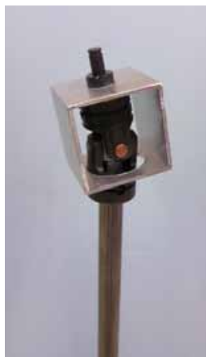
Fig. 6.9:Connector consisted of universal joint and ball bearing.
