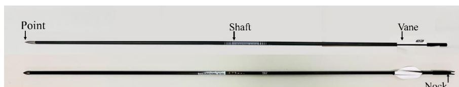
Fig. 2 Arrows shot by the shooting machine (upper: A/C/E shaft, Diamond vanes, and streamlined point) and by the robot (bottom: X10 shaft, Spin-Wing-Vanes, bulge point, and In-Out nock).
