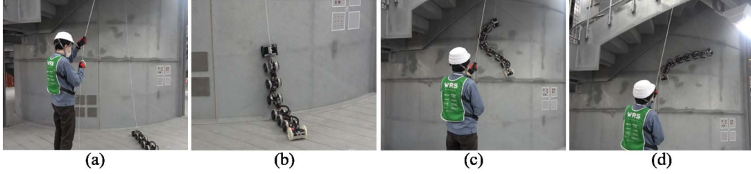
Figure 17. Result of the experiment of moving on a large tank at the World Robot Summit 2020.
