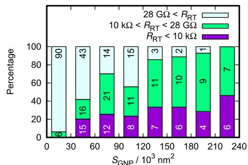
**Fig. 7**  $R_{RT}$  distribution classified by  $S_{GNP}$  for  $f_{DEP} > 20 \text{ kHz}$ . Numerals in bins represent the number of corresponding electrode pairs.
