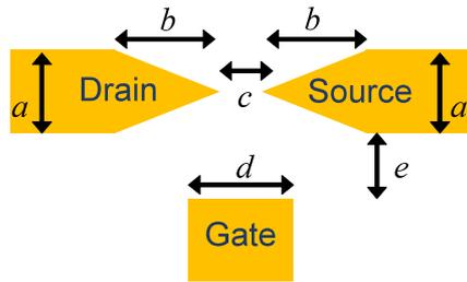
**Fig. 1** Schematic illustration of electrodes (top view). An AC voltage was applied between the source and drain electrode. The dimensions are as follows.  $a$ : 800 nm,  $b$ :  $1.2\ \mu\text{m}$ ,  $c$ : 100–200 nm as the target value (actually fabricated in the range of 100–400 nm),  $d$ : 500–900 nm,  $e$ : 0– $1\ \mu\text{m}$ .
