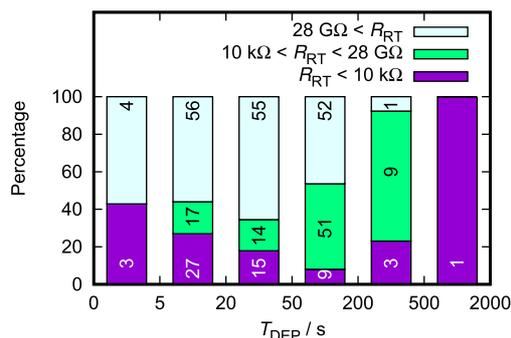
**Fig. 5**  $R_{RT}$  distribution classified by  $T_{DEP}$  for  $f_{DEP} > 20 \text{ kHz}$ . Numerals in bins represent the number of corresponding electrode pairs. Note that the  $T_{DEP}$  regions on the horizontal axis are not equally divided.
