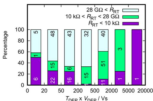
**Fig. 6**  $R_{RT}$  distribution classified by the product of  $T_{DEP}$  and  $V_{DEP}$  for  $f_{DEP} > 20 \text{ kHz}$ . Numerals in bins represent the number of corresponding electrode pairs. Note that the  $T_{DEP}V_{DEP}$  regions on the horizontal axis are not equally divided.
