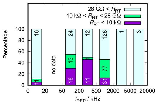
**Fig. 3**  $R_{RT}$  distribution classified by  $f_{DEP}$ . Numerals in bins represent the number of corresponding electrode pairs. Note that the  $f_{DEP}$  regions on the horizontal axis are not equally divided.
