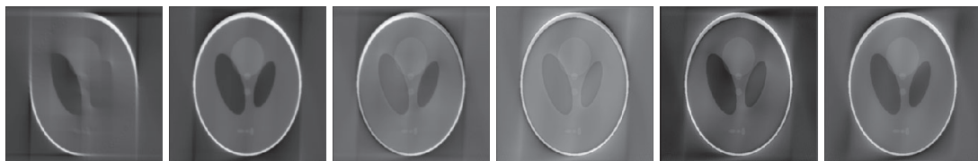
Figure 10: Reconstruction of a phantom by the SART method
