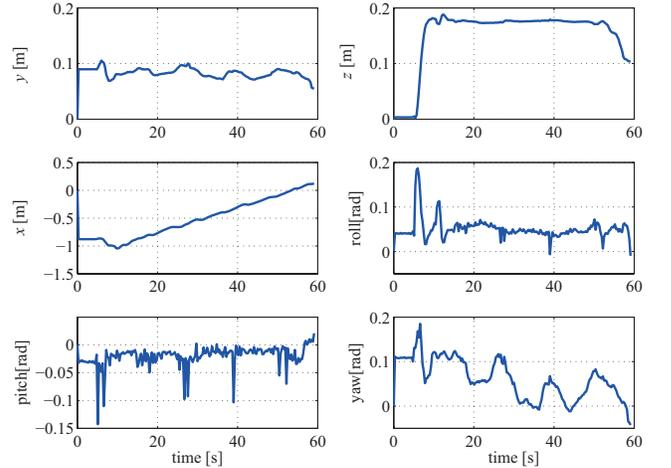
Fig. 17. Time response of the head position of the snake robot.
