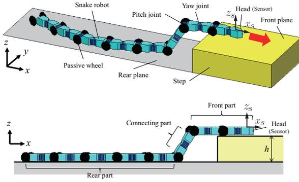
Fig. 2. Snake robot landing on the front plane of a step.
