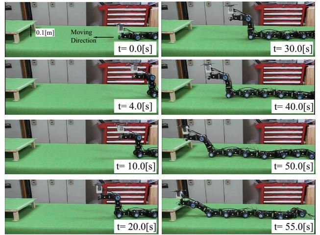
Fig. 12. Snapshots of a typical step climbing experiment.
