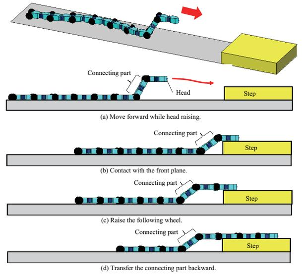
Fig. 4. Head raising of a snake robot in approaching the step.
