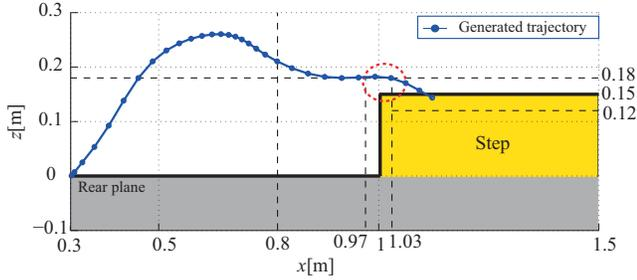
Fig. 10. Generated trajectory using our method with transition constraints.
