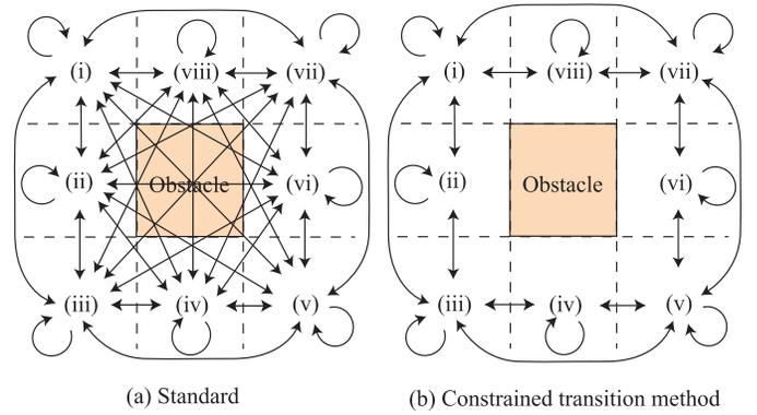
Fig. 8. Transition condition for the obstacle avoidance constraint.
