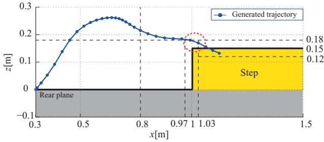
Fig. 9. Generated trajectory using our method without the transition constraint.
