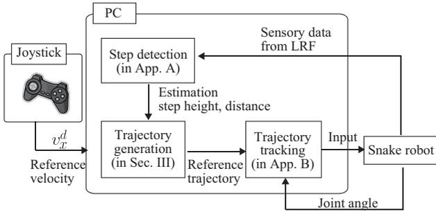
Fig. 7. Outline of the propose system including the trajectory generation method.
