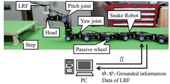
Fig. 11. Photo of the experimental system.
