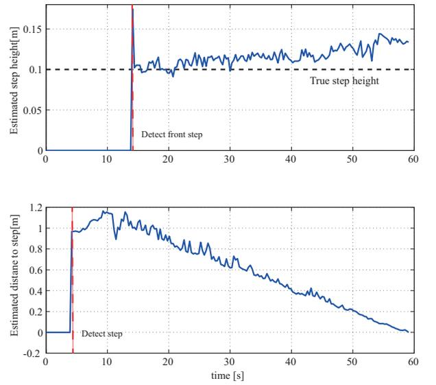
Fig. 16. Estimation of the step height.
