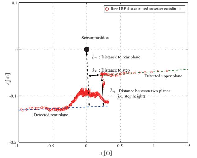
Fig. 20. Example of step detection. Distances to front and rear planes are estimated.
