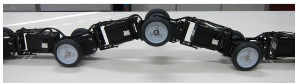
Figure 17. An example of lifting motion of the snake robot by pitch joints.
