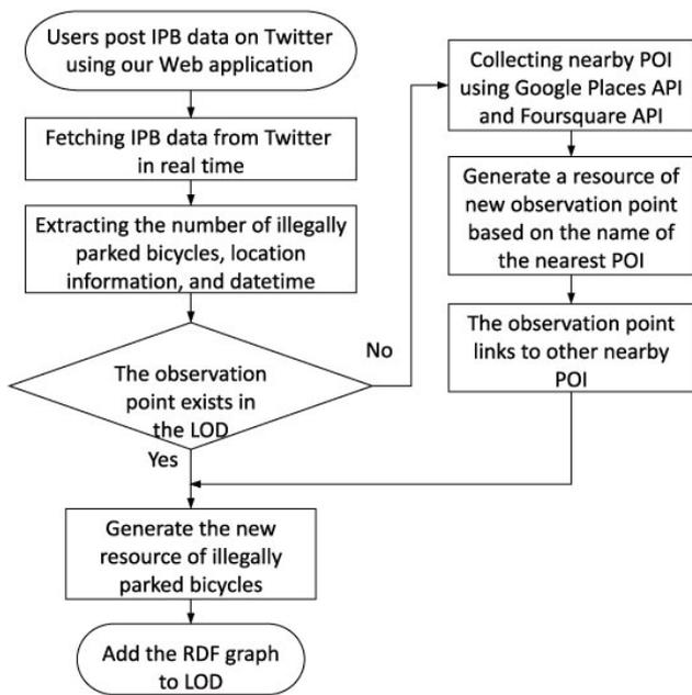
Fig. 4 Procedure of LOD building
