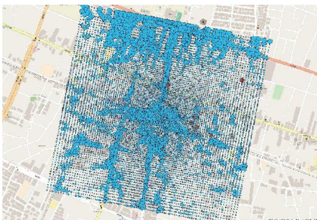
Fig. 9 The result of the airflow simulation. (The size of blue circle is the average wind velocity. Red markers are observation points.)
