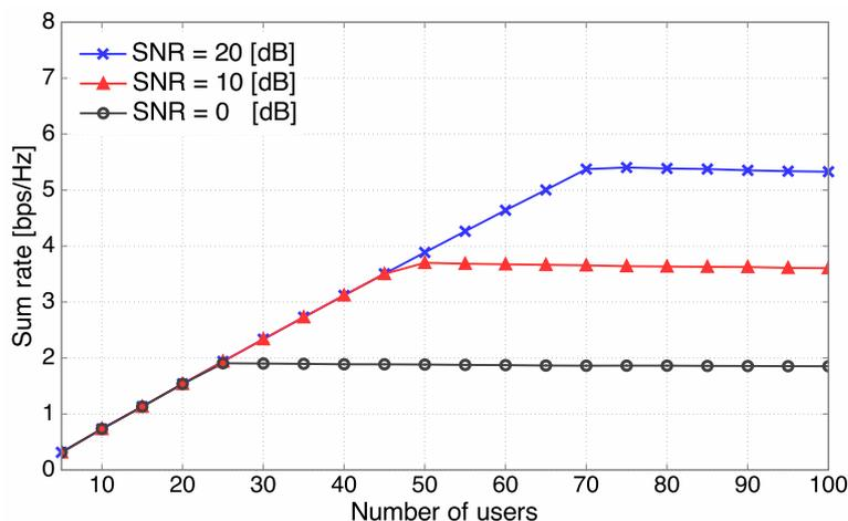
**Figure 4.2: Sum rate performance for various number of users - using the proposed power allocation algorithm.**
