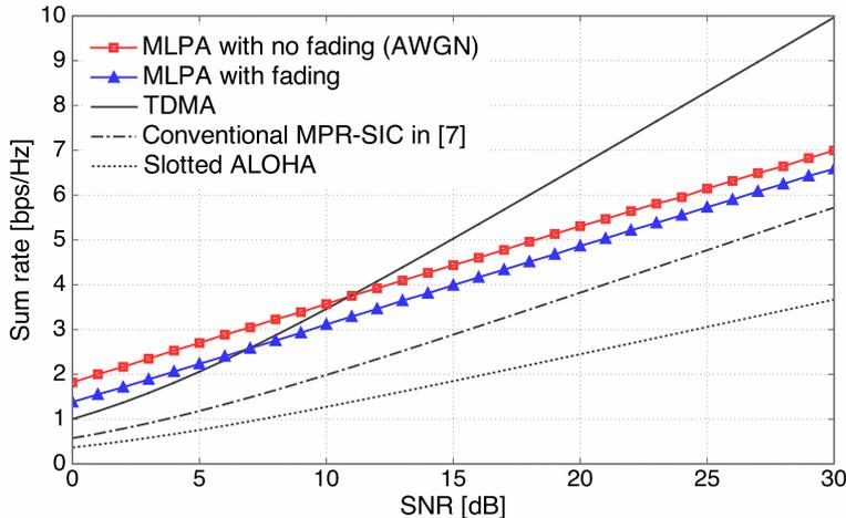
**Figure 4.1: Sum rate performance of various schemes for the AWGN channel - with  $K = 100$ .**
