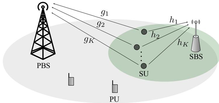
**Figure 5.1:** The random access system model of the CR network - with  $K$  SUs, one SBS, and one PBS.
