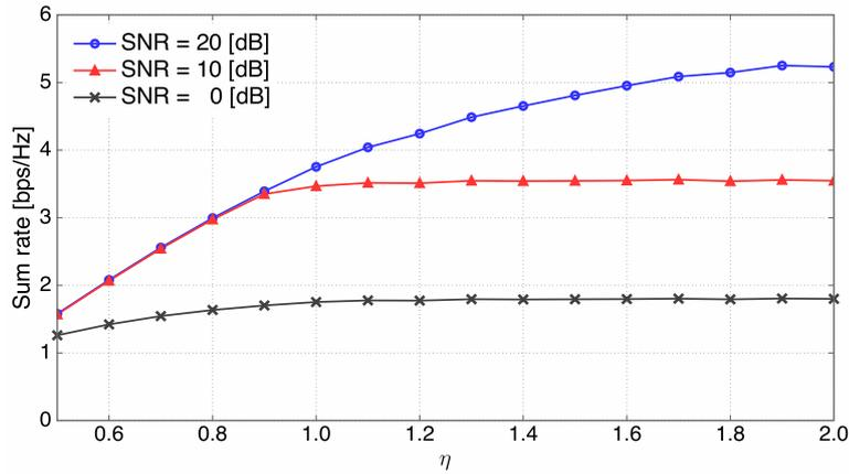
Figure 5.5: System sum rate according to  $\eta$  using the proposed DPA and OTP - for various values of SNR.
