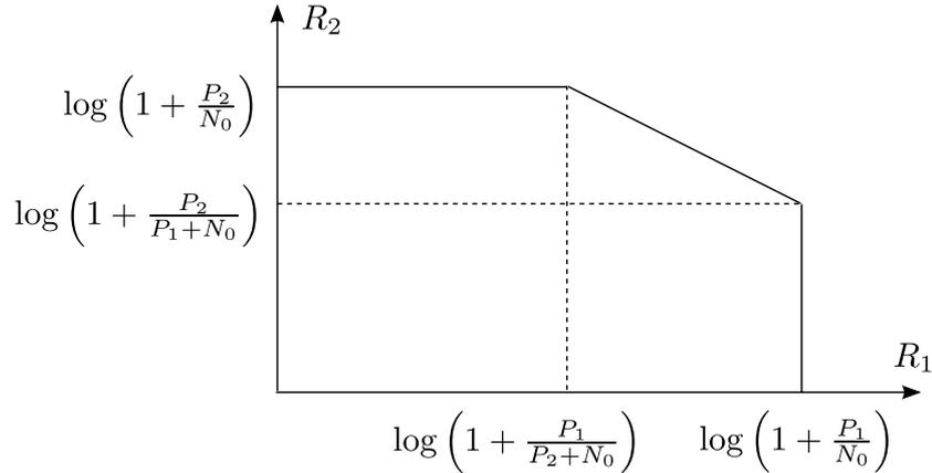
**Figure 2.3: Capacity regions of two-user Gaussian multiple-access channel** - can be achieved by the SIC decoding.
