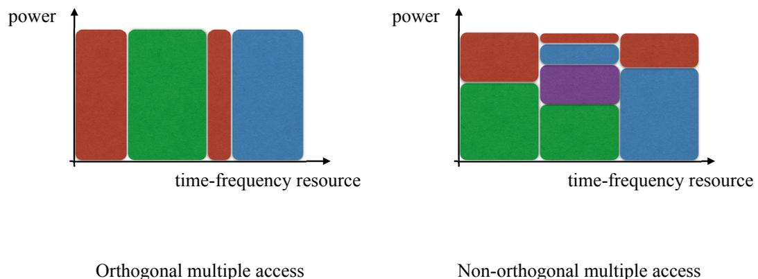
**Figure 1.1: Comparison of OMA and NOMA** - non-orthogonal power division vs. orthogonal time-frequency division.
