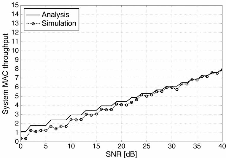
**Figure 3.6: Analytical and simulated throughput of the random access system with the decentralized multilevel power allocation - for various  $1/N_0$  values with  $K = 100$  and  $\Delta = 0.1$ .**
