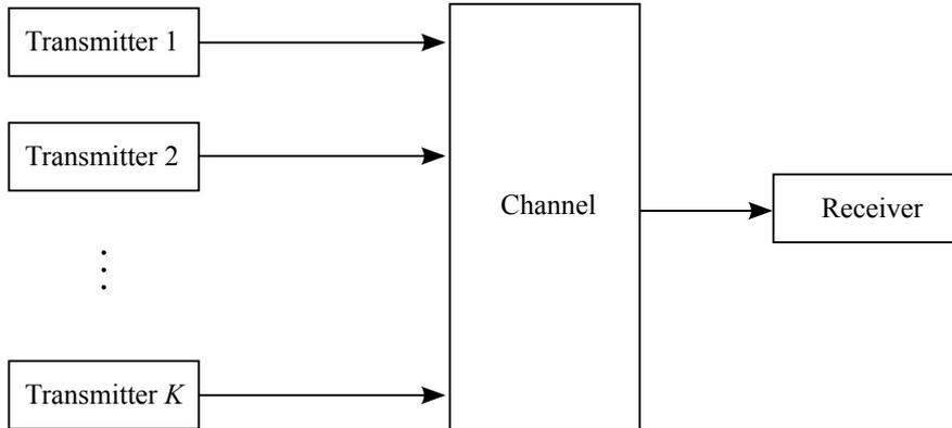
**Figure 2.1:** Block diagram of the multiple access system - with  $K$  transmitters communicating to one receiver.
