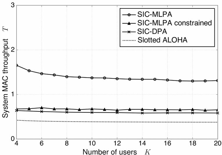
**Figure 3.7:** Comparison of system MAC throughput for the AWGN channel - for various schemes with different numbers of users.
