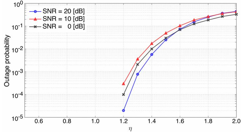
**Figure 5.7: Outage probability of the interference temperature at the PBS according to  $\eta$  - for various values of SNR.**
