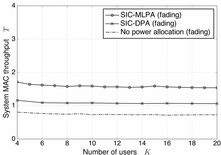
**Figure 3.8: Comparison of system MAC throughput in the fading environment** - for various schemes with different numbers of users.
