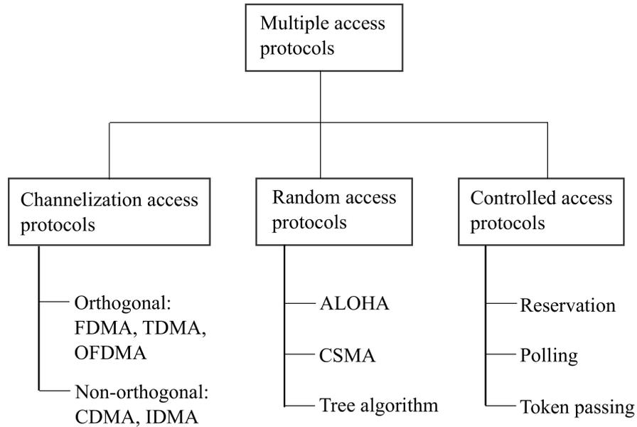
**Figure 2.2: Taxonomy of the multiple access protocols** - channelization access, random access, controlled access.
