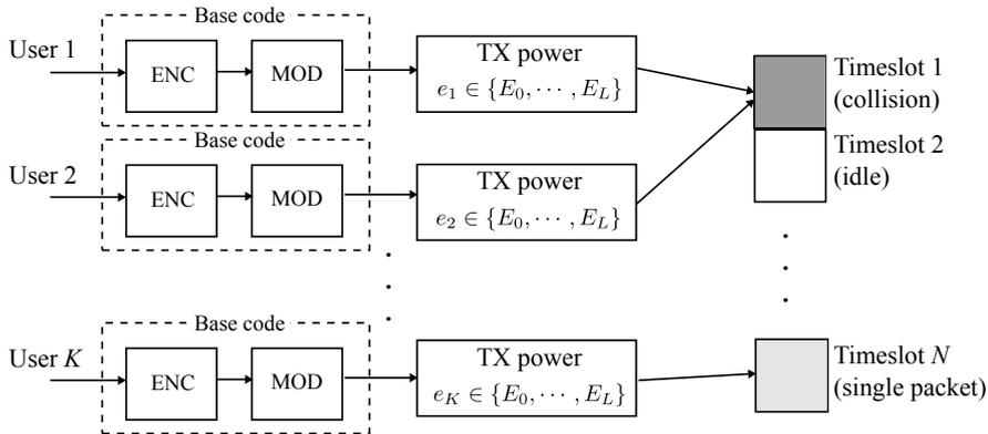
**Figure 3.2:** Block diagram of the random access system using decentralized power allocation - using the same base code, with  $K$  users during  $N$  time slots.
