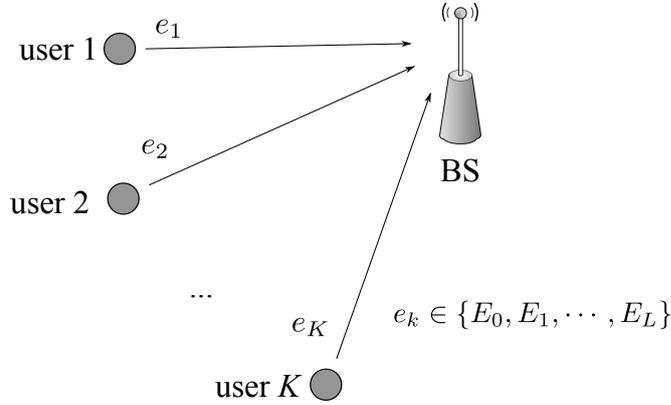
**Figure 3.1:** System model of the random access system using decentralized power allocation - with  $K$  users and one common BS.
