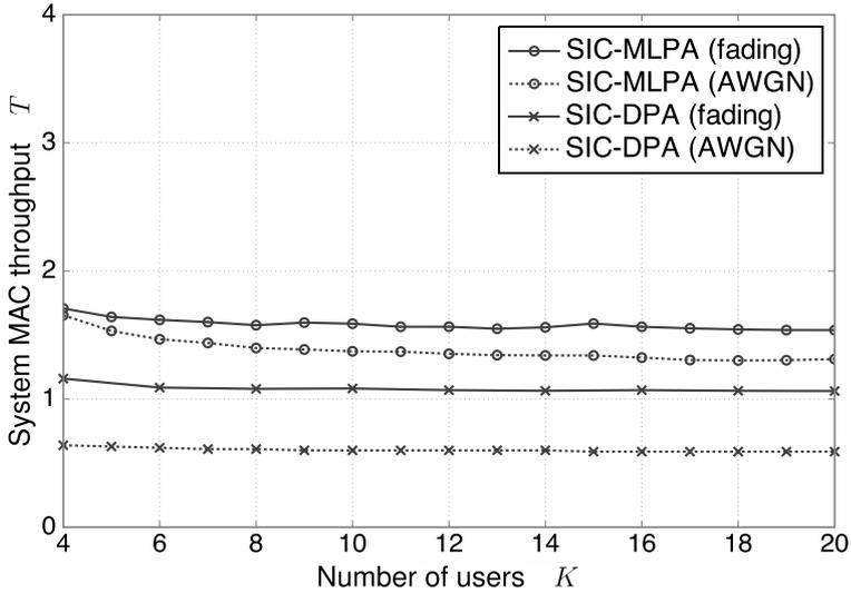
**Figure 3.9: Comparison of system MAC throughput in the AWGN environment and in the fading environment - for various schemes with different numbers of users.**
