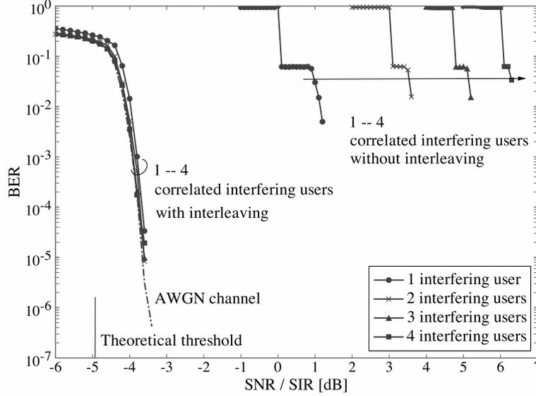
**Figure 3.3: Bit error rate performance of the scheme with totally correlated interfering users, using BICM or not using BICM - a turbo code with component code of rate 1/3 RSC code  $(15, 17)_8$  in octal form is used. The information size is 1530 bits and quadrature phase shift keying (QPSK) is used.**
