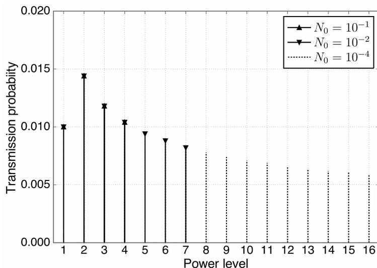
**Figure 3.5: Obtained probabilities according to various noise power levels** - The abscissa axis stands for the index of power levels ( $E_1, E_2, \dots, E_L$ ). Note that the sum probability shown in this figure is less than 1, since the power level  $E_0 = 0$  (no transmission) is not shown there. In the system, the sum probability of all power levels from  $E_0$  to  $E_L$  is 1.
