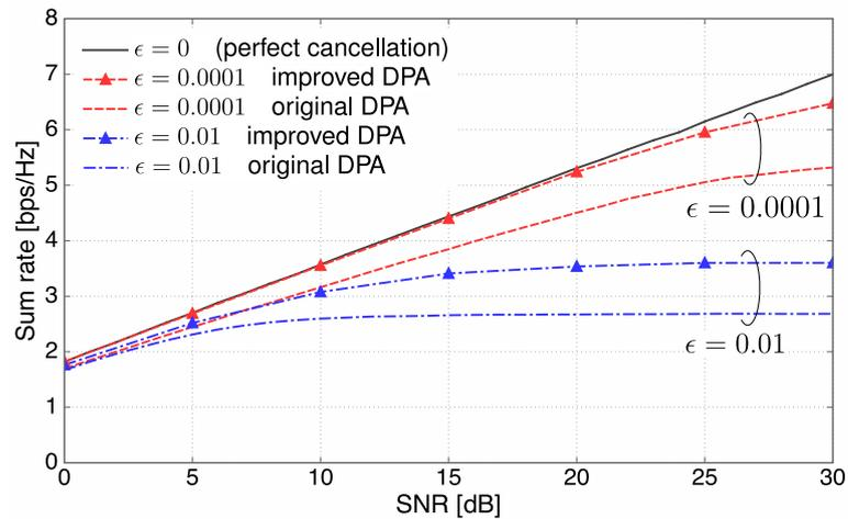
**Figure 5.4: Comparison between the original DPA and the improved DPA - for various values of the cancellation residual ratio  $\epsilon$ .**
