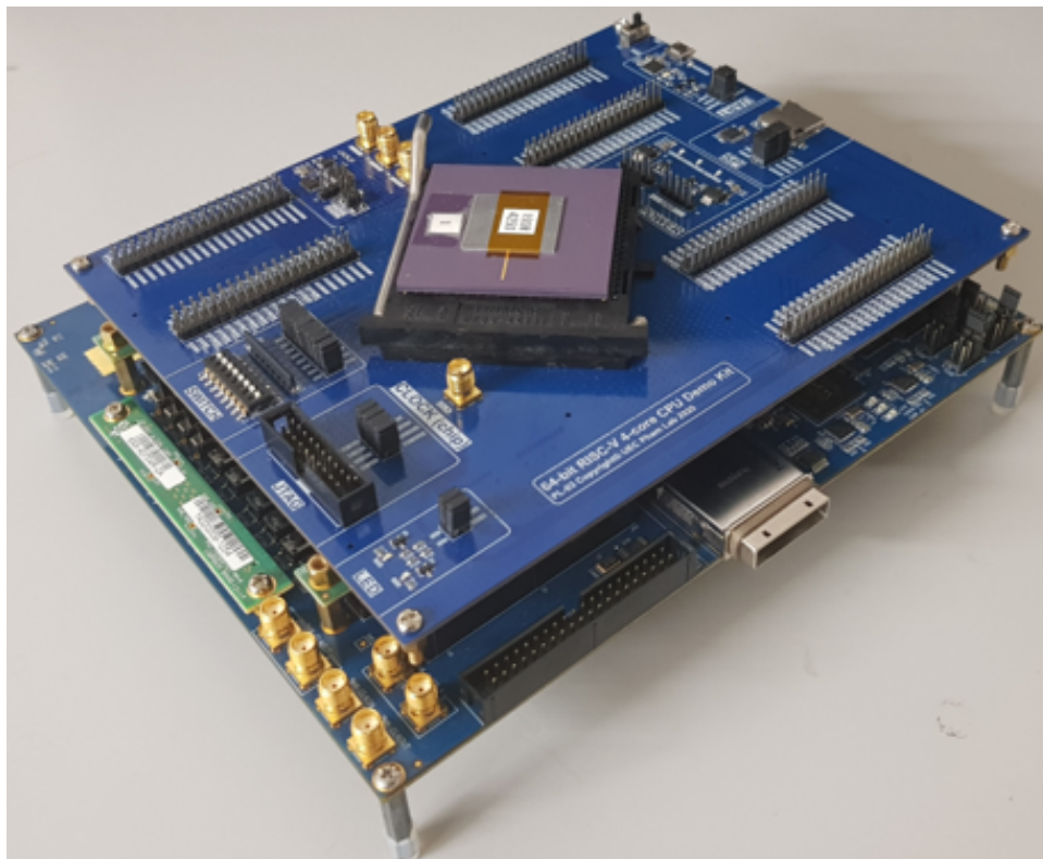
FIGURE 3.35: The quad-core Rocket-computer PCB mounts on the TR4 FPGA board.
